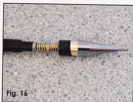
Test-fitting the insert; the tip should screw down and hold it firmly.
