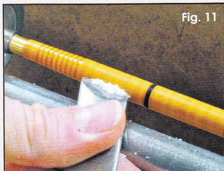
Before polishing, scrape the CA lightly with the skew to level it.
