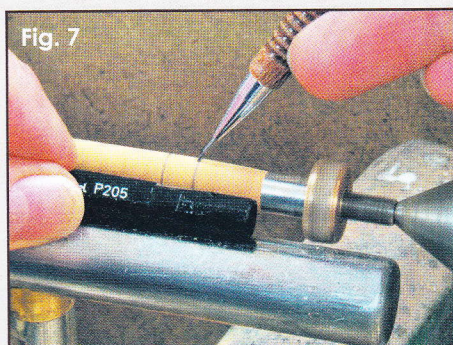
Use the original sleeve to mark off the clip recess.
