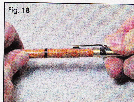
The clip jig is shown in action; push the end of the clip only.
