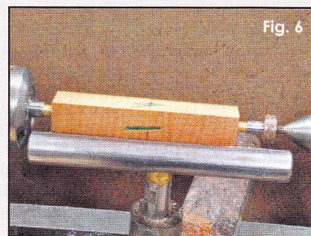
The blank is mounted and ready for turning.
