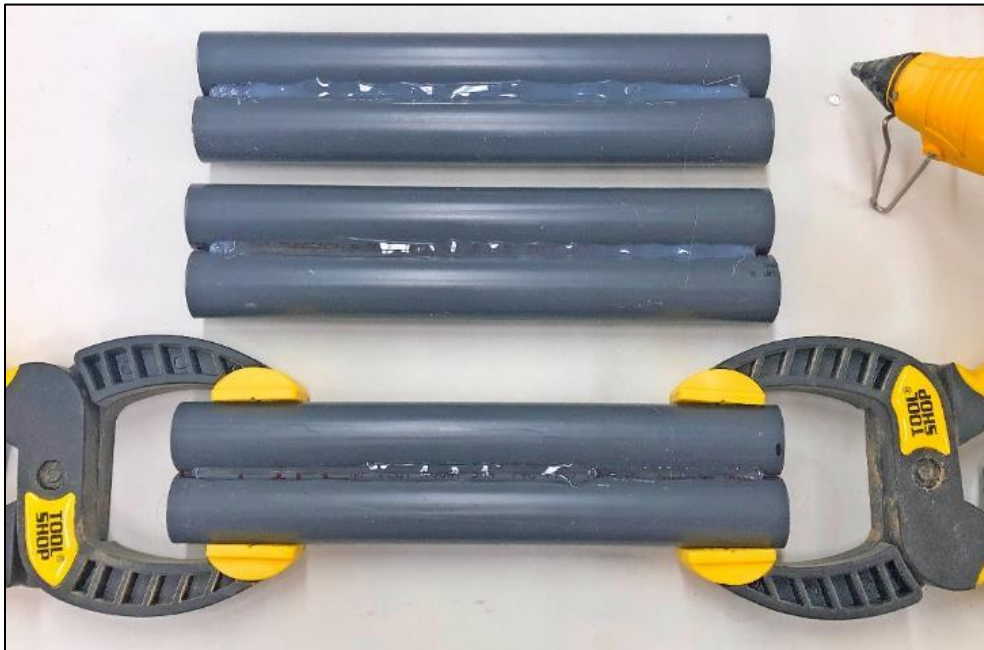
Figure 3. Six pieces of Pipe each 8\frac{3}{4} " inches long made into pairs using hot melt glue.
