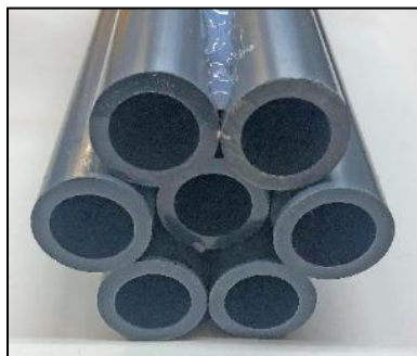
Figure 6. The final pair glued onto the assembly to complete the mold.
