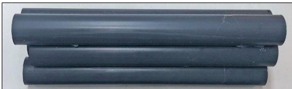
Figure 5. Another pair glued on keeping the shorter tube in the center.
