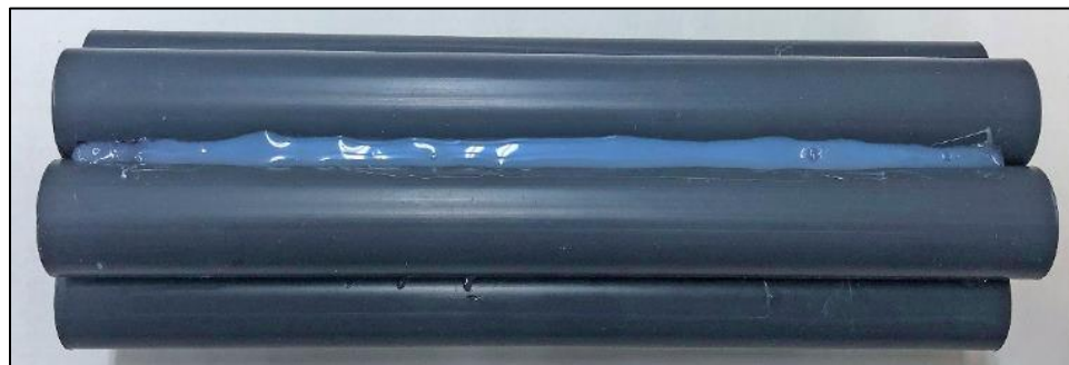
Figure 6. The final pair glued onto the assembly to complete the mold.
