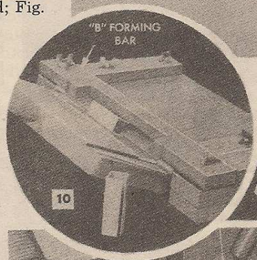
MAKING A CHANNEL WITH STYLE "B" FORMING BAR
