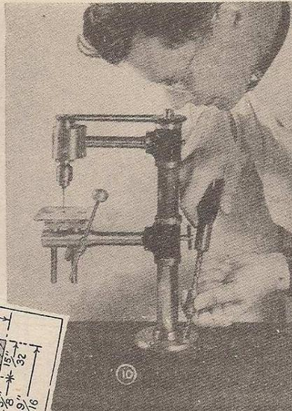
back, while a larger one of brass is fitted in the other tee for adjusting the table.
