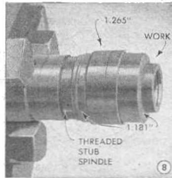
First the work is mounted on a threaded stub spindle. Then major and minor diameters are turned
