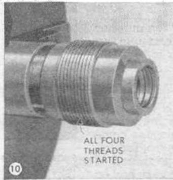
Engaging the dial as outlined produces four starts which are finally deepened to finish the threads
