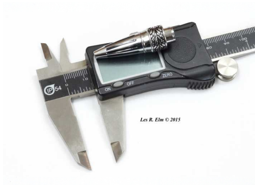
Nib Section Measurement at 0.495"
