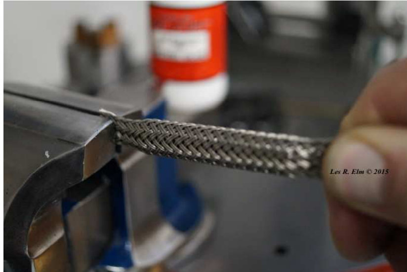
Holding Tension on the Nylon Braid
