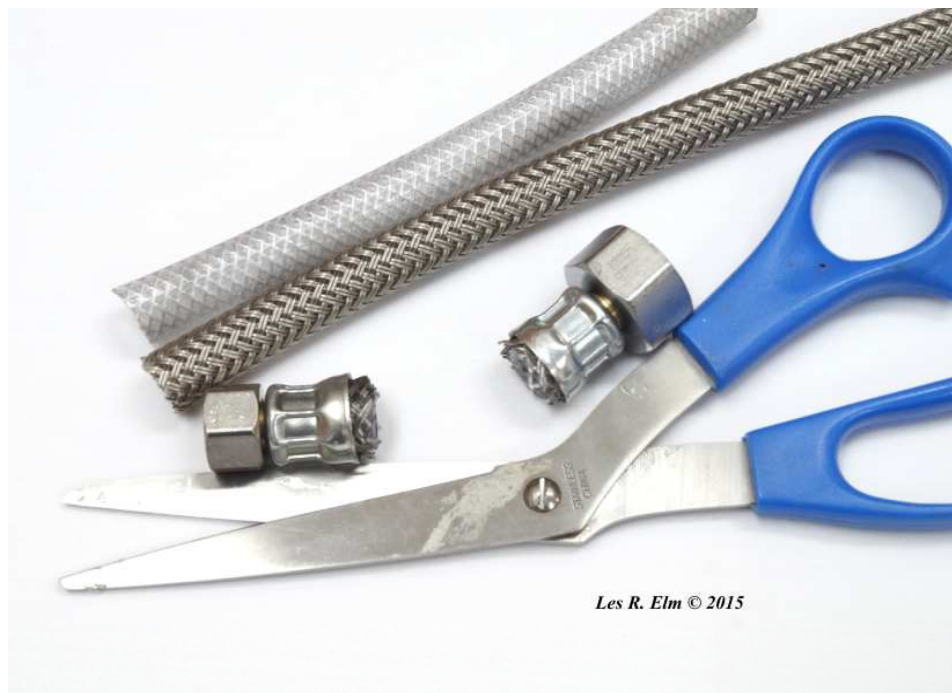
Connector with fittings and tube remove
