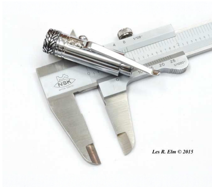
Finial Section Measurement at 0.495"
