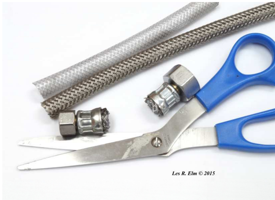
Connector with fittings and tube remove
