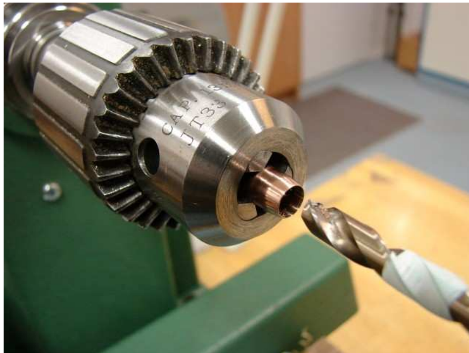
Bullet Drilled to a Depth of 3/4" with a 1/4" Bit
