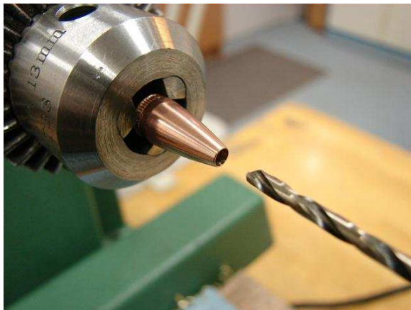
Drilled #36 Nib Hole
