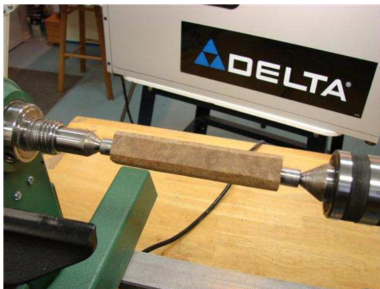
Turning Between Centers with Bushings
