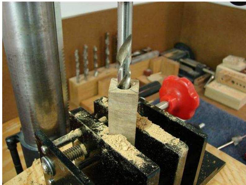
Drilling the Blank Through From One End
