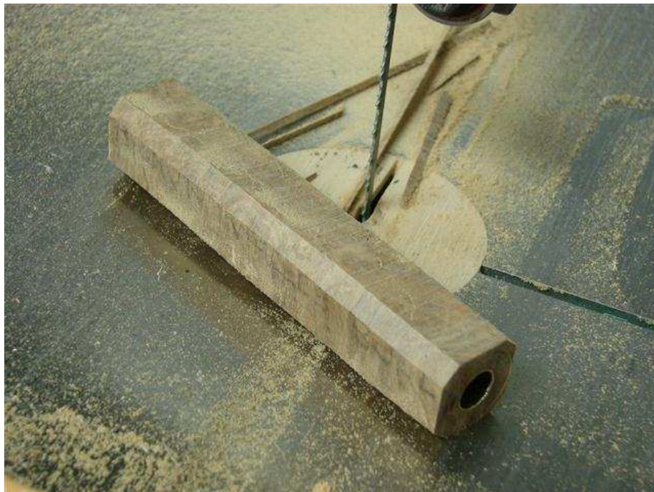
Remove The 4 Corners Off The Blank
