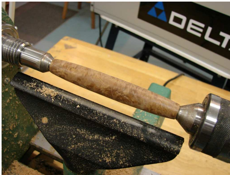
Blank Turned Down and Shaped Proud of Bushings
