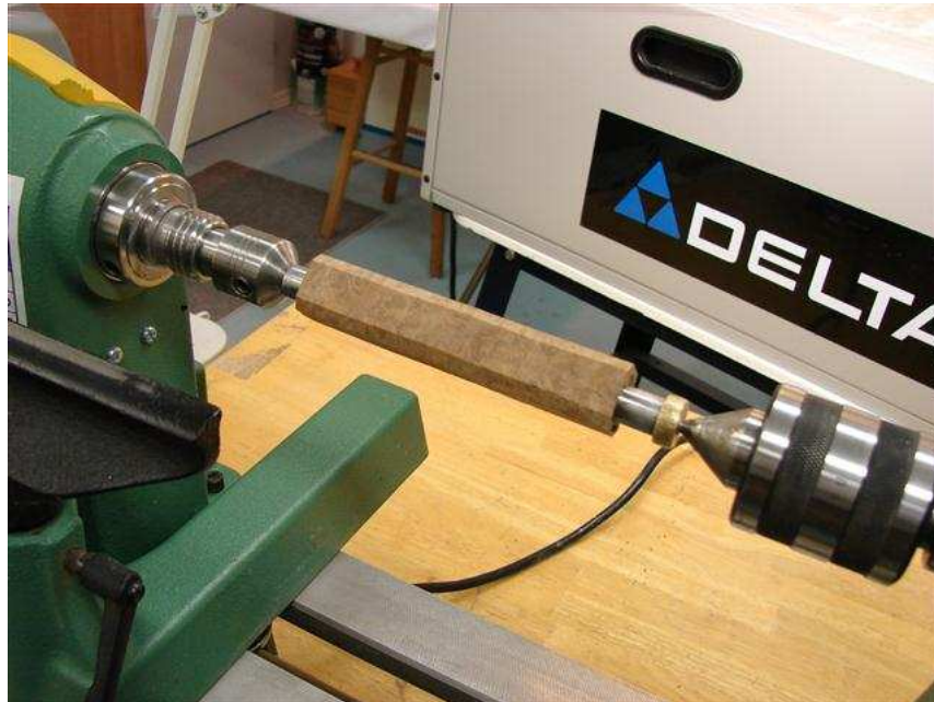
Mandrel Turning with Bushings
