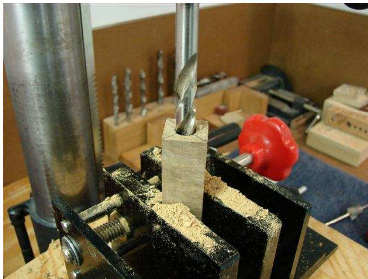
Blank Drilled to Depth with 27/64ths Bit
