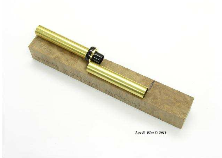
Mark the 3/4" Blank to Cut at 4-1/2"
