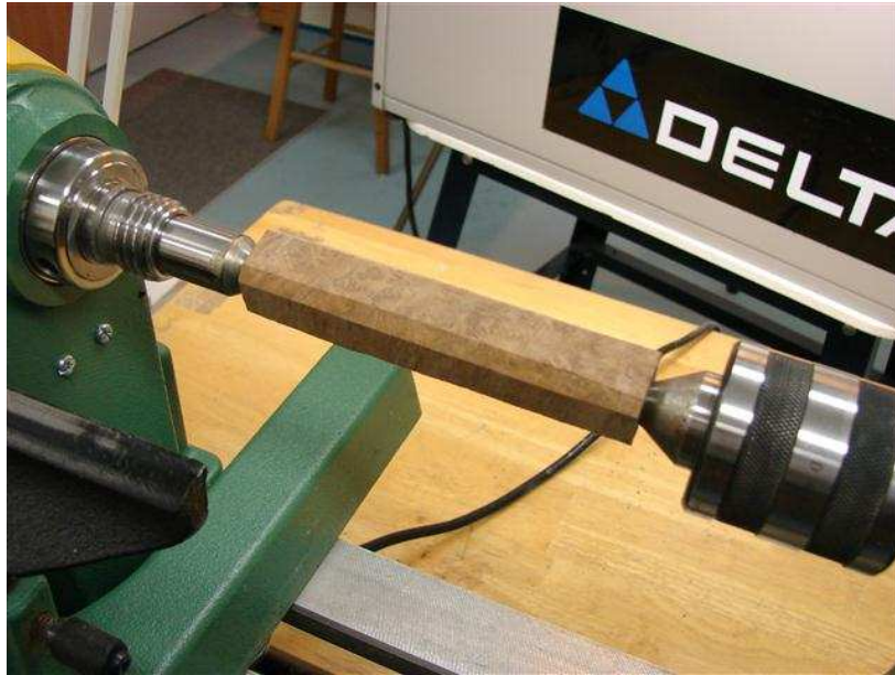
Turning Between Centers Without Bushings
