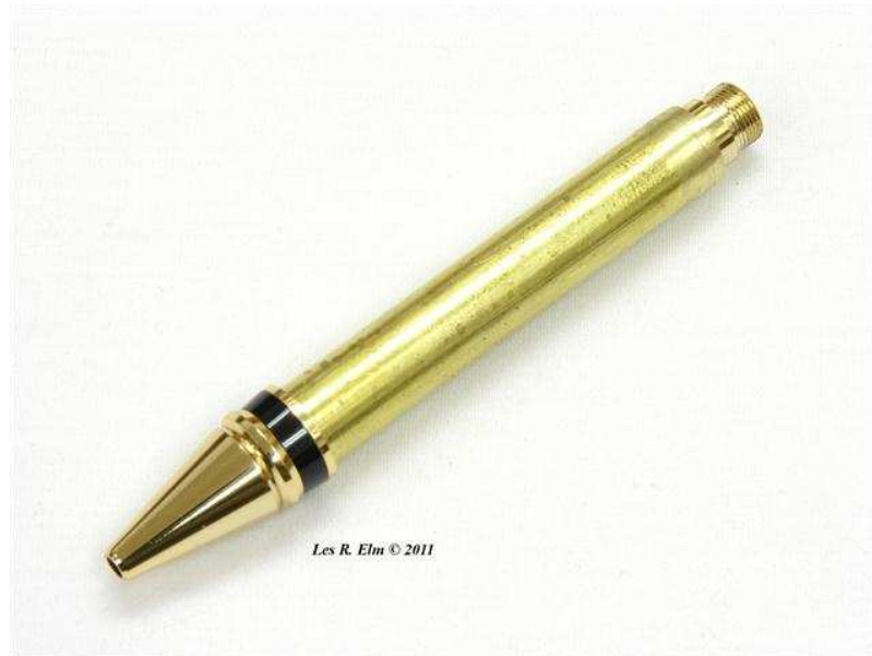
Nib Installed on Lower (Long) Tube
