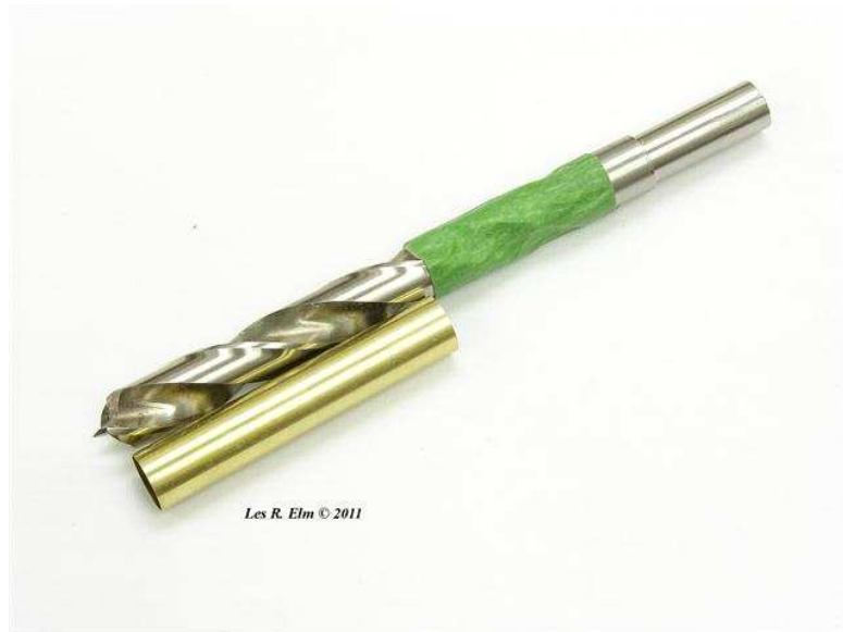
Drilling Depth Marked on 27/64ths Drill Bit
