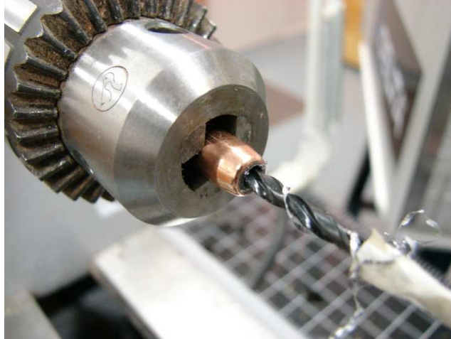
Drilling 9/64ths Bullet Nib Hole
