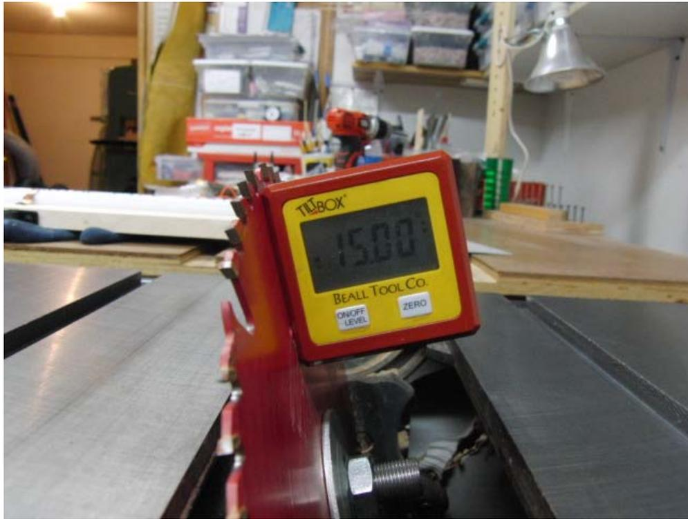
Photo 9 – in this photo the 7 ¼" blade is installed. Line up the wood to make the first cut which will be a throw away. Do not worry about the Rockler jig yet. **Please note at this time the shopvac is now turned on.**
