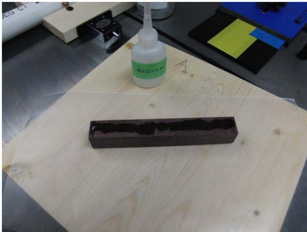
Photo 22 – the CA is cured. The blank is on the sacrificial piece good and solid now
