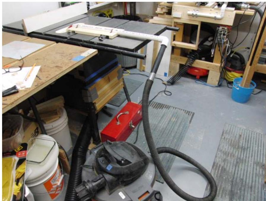
Photo 2 - The jig consists of a piece of 1" PVC pipe strapped down on a "dadoed" piece of 3/4" pine that can be positioned (related to the saw blade) and it is held down by 4 on/off magnets.
