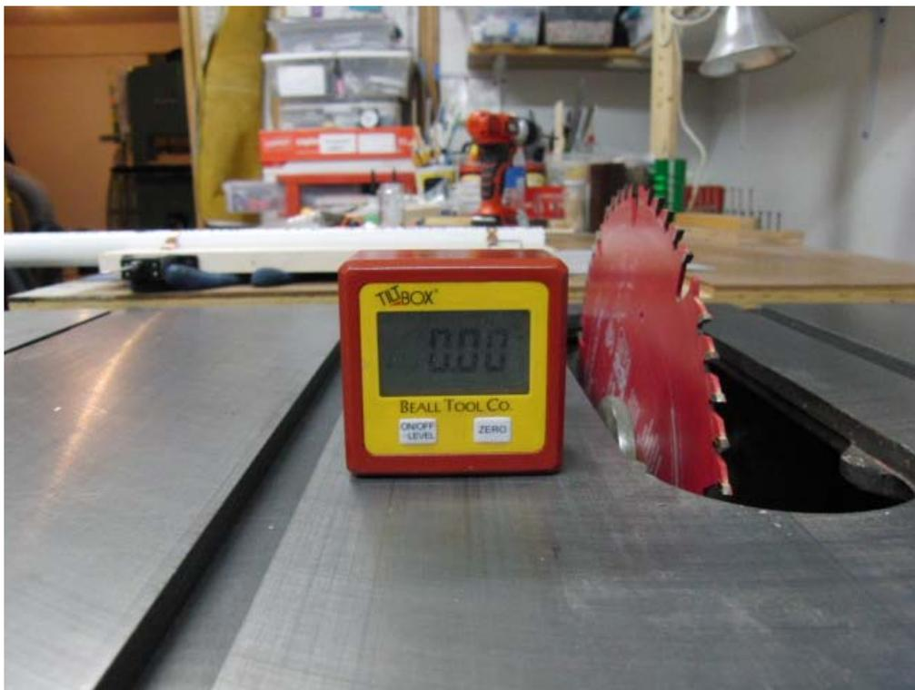
Photo 8 - I find using the 10" blade is easier and more accurate to achieve the 15 degrees. Once you have angle you want, remove the 10" blade and install the 7 ¼" blade.
