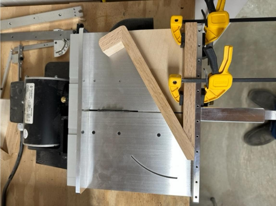
Hold your pen blank, which will be the main body, against the stop, making sure the blank is just past the blade and make that cut.
