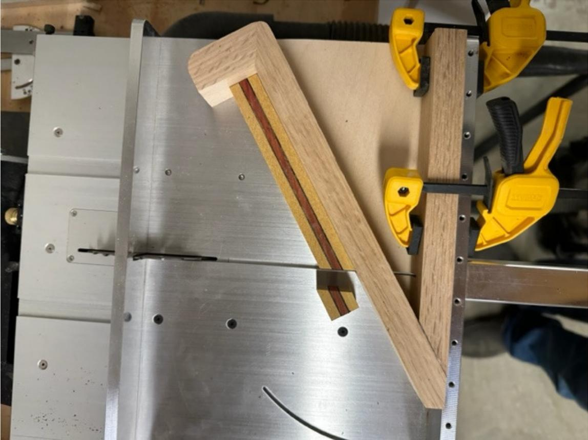
Rotate the blank 180 degrees and make the same cut. The point will automatically be centered on the blank.
