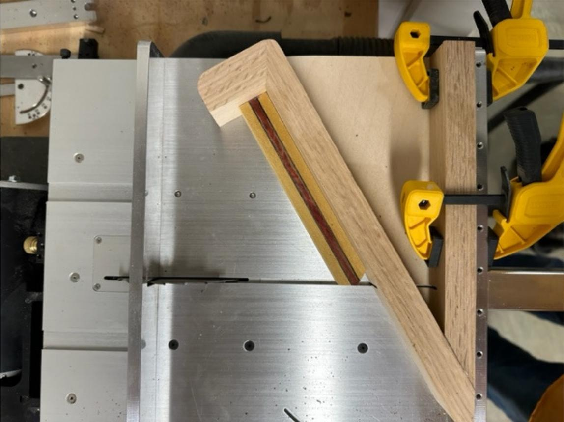
If you desire, you can now put a spacer between the 90 degree stop and the pen blank and make the exact same cuts on the opposite end. This is where an adjustable stop would come into play; I opted to just use a spacer.
