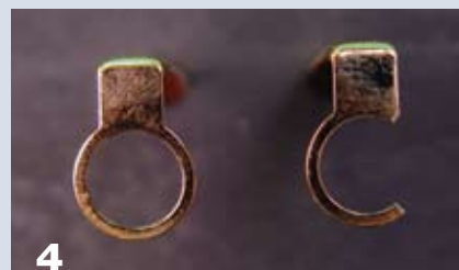
4 If the ring fits inside the cap tube, the only modification is to remove a section of the ring so it may be threaded to the inside of the cap, as with this El Grande clip in a Baron cap tube.
