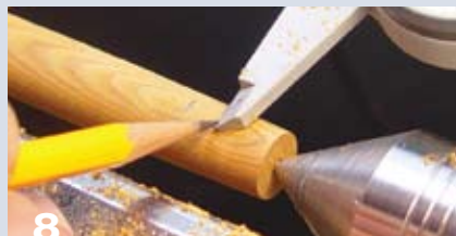
Mark the location of the clip slot and the end of the pen.
