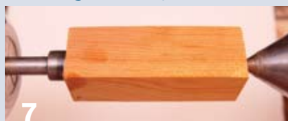
Put the drilled blank on the mandrel and turn to shape. Shown is a blank screw onto a standard 7 mm mandrel that is held in a collet chuck. The tailstock center is just there for additional support, and is not required to drive the blank.
