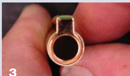
3 Using the brass tube as a sizing gauge, the ring must fit inside of the tube, as the El Grande shown here with the Baron cap tube.
