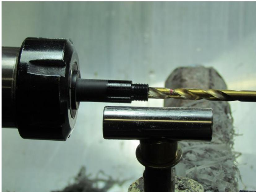
Since I have no drill bit the right size to provide a snug fit for the converter I follow the drilling with a .252" reamer which only goes in enough to allow the converter to seat itself.
