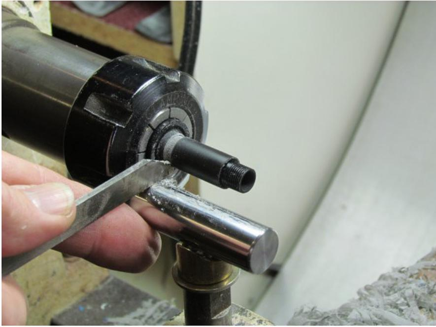
I change collets for the first time switching to one that fits the finished diameter of the section then insert the section in threads first.
