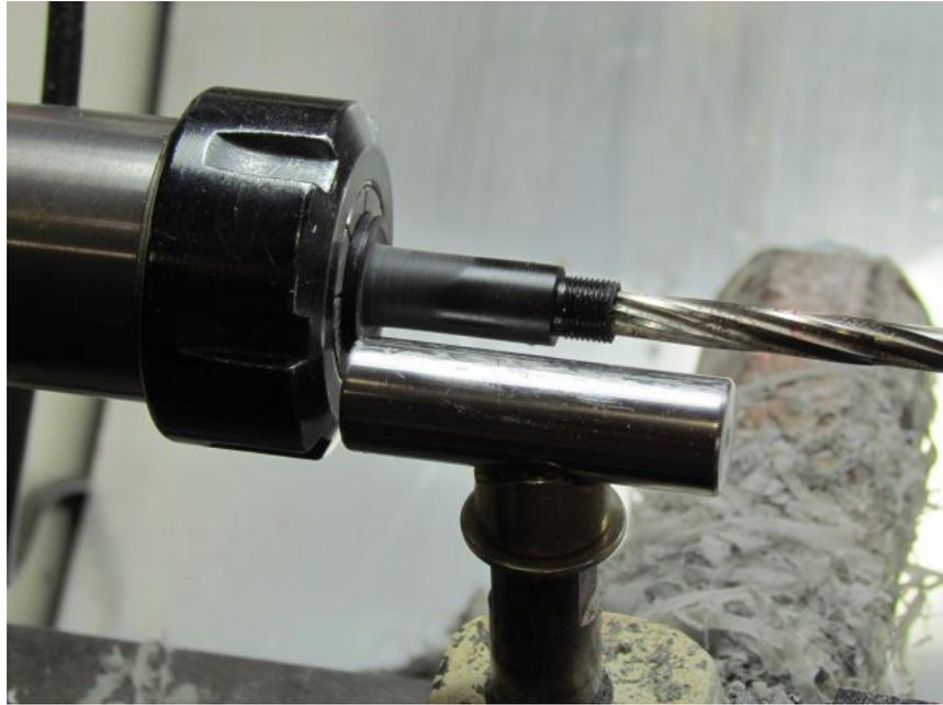
Seating the converter snugly but NOT too tight is important. Too loose and the converter will fall off into the pen and would probably make a mess, too tight and you'll likely crack the section since this a fairly delicate part of the pen. Don't go any further unless this fits like a glove!
