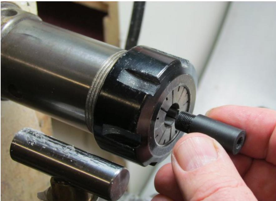
Now I drill a hole in only far enough to allow the smooth portion of the feed housing to easily slide in but not so far as to destroy the section I am going to thread next.
