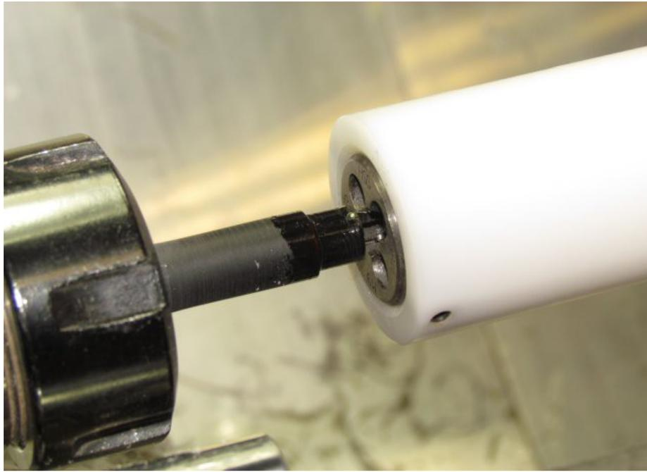
Here I am actually cutting the threads using a die holder which spins freely on a rod that is chucked into the tailstock
