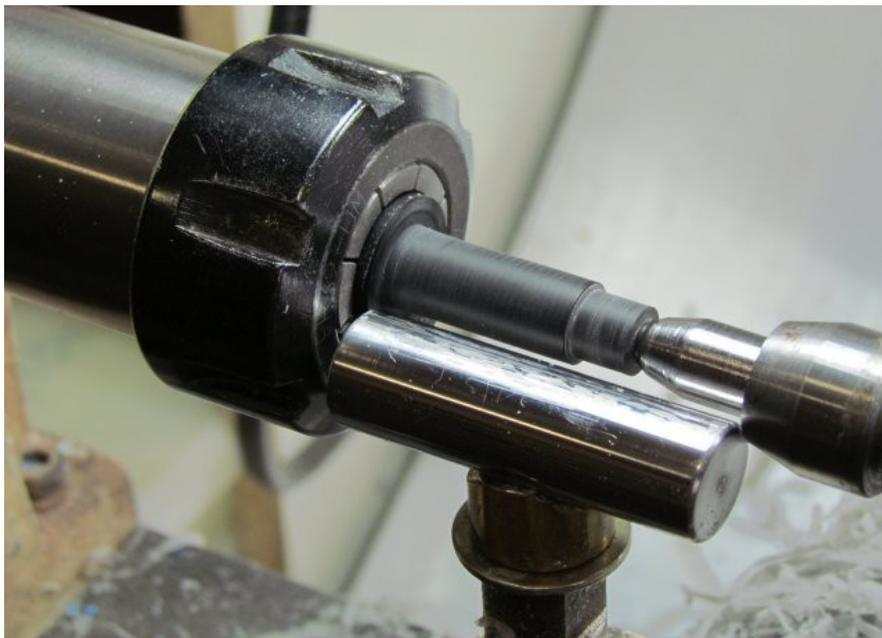
I spray a bit of cooking spray such as PAM to lubricate the blank and proceed to thread the section. Why cooking spray... why not! I like it because I can spray a tiny quick shot on the blank then a quick shot into the die then it cleans off easily after use.
