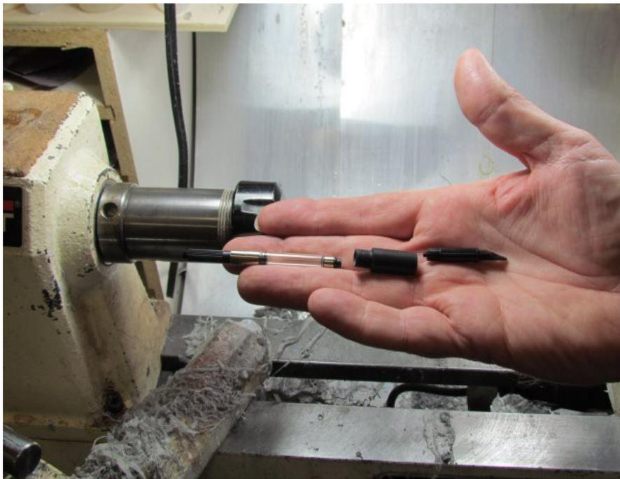
Here is the section with the converter inserted, the feed housing screwed in and the feed itself inserted into the housing. Well there's my pen, all you need now is a little ink in the converter, a nib on the feed and you're in business! But most folks want something
