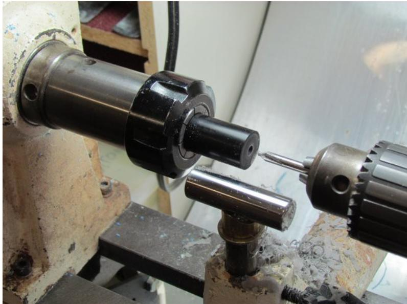
Here the blank has been turned down to the approximate finished size and a tenon for the rear threads has been turned. Look closely at the tool rest, I applied a bit of ski wax because I want my tools to slide freely on the rest while making delicate cuts. Any "non sticky" wax will work.
