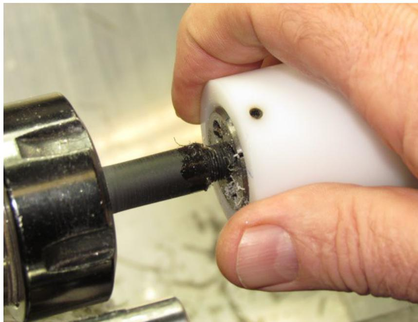
After threading, take a narrow parting tool and clean up the threads at the end closest to the section body so it will thread flush to the pen body (Look closely to the left of the threads to see the area cleaned up). Now I drill the first hole as deep as I want the section to be, in this case 1.1" long. This is the drill size used for whatever tap you select so choose it carefully. The second drill I use is to allow the fountain converter to fit inside the section as shown a few photos down.
