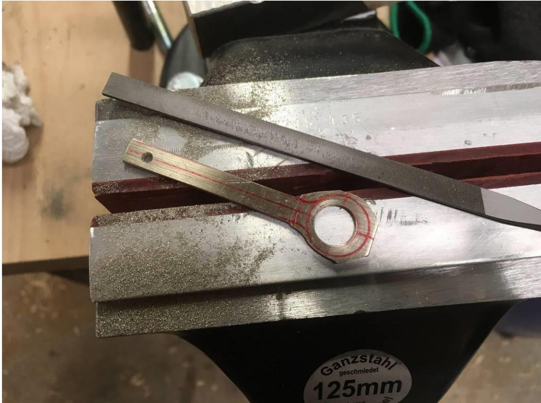
For the radius, I turned a template with the finished outer diameter.
