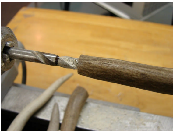
Drilling up to Depth Mark
