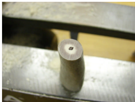
Drill Bit Exit Mark
