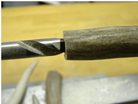
Stop Drilling at Depth Mark
