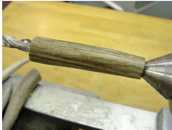
Antler Reversed to Finish Drilling Hole
