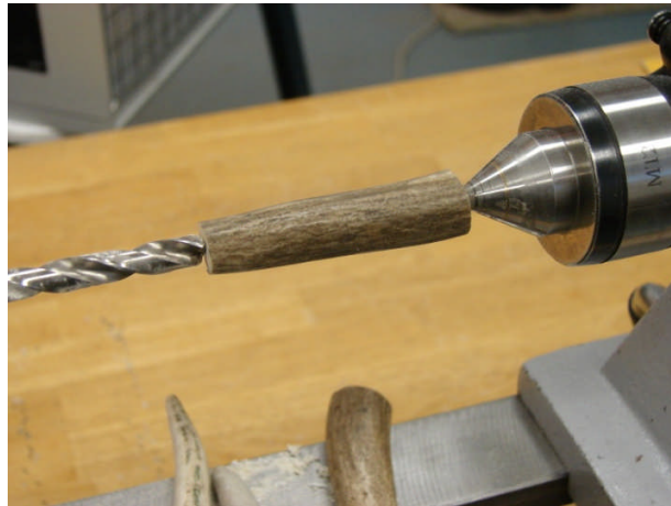
Antler Blank Installed Between Bit and Live Center
