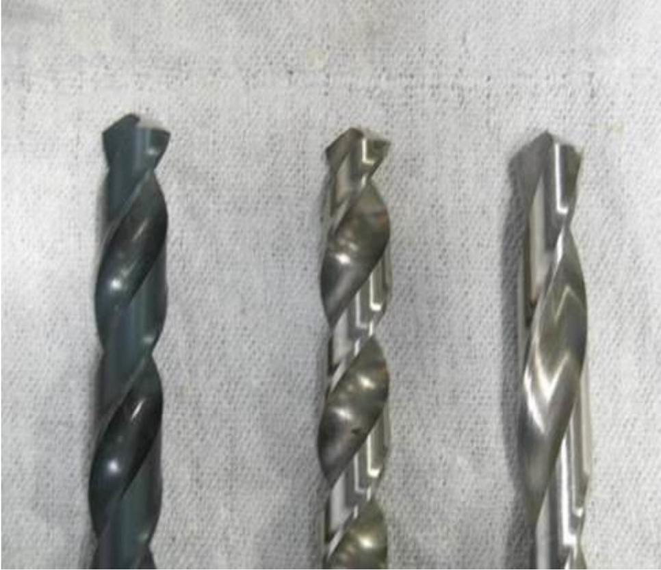
The helix angle of drill bits is not a standard. Helix angles vary from slow (not many turns per inch) to fast (lots of helical spirals going up the bit). Bits sharpened at the same setting will have remarkably different chisel and relief angles.
