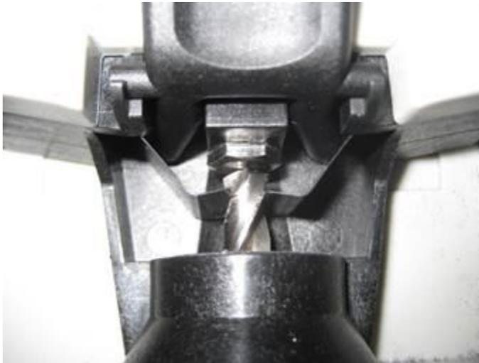
4. If you are sharpening 118° drill bits, make sure you have your sharpener set at 118°. If you are sharpening 135° drill bits, make sure you have it set at 135°.
