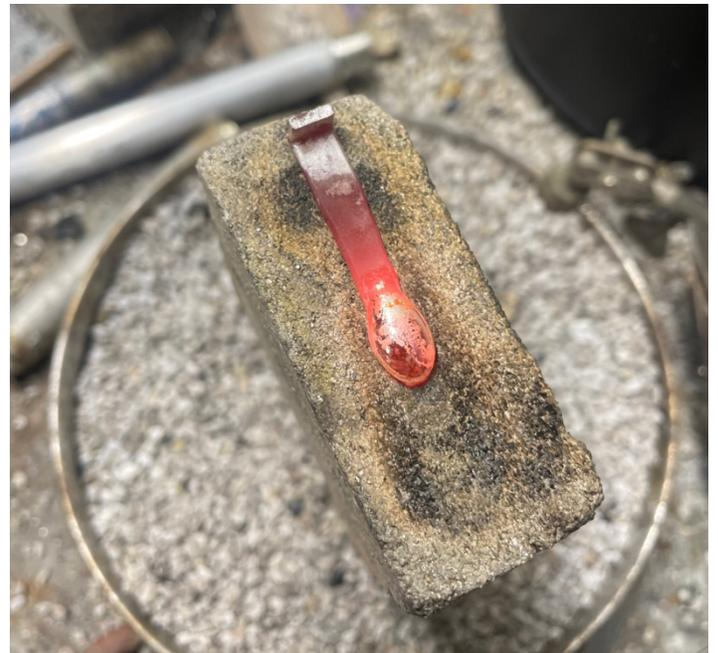
Now I use a hammer and bench block to shape the end of the clip so it tapers with the rest of the clip. The clip is still wonky, so it needs to be refined with files and some hammering.
