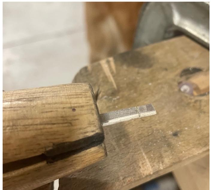
I then use a triangular file to hog the metal out down to where the cut stops, then switch to a square file to finish.
