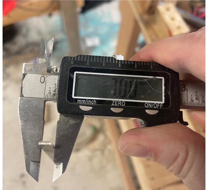
Now it's time to put the bend in the clip where it will be soldered to the clip ring. I begin by trimming the end off, and then scoring a line mostly through the clip with a jeweler's saw.
