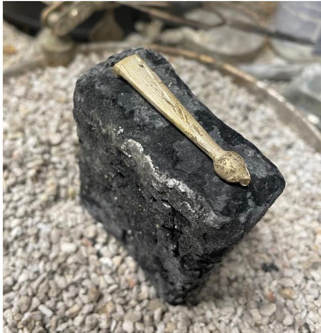
I begin by bringing the clip to its melting point, where the metal starts to ball up and flow together. Left pic is the cooled clip. I don't worry about it being wonky at this point.
