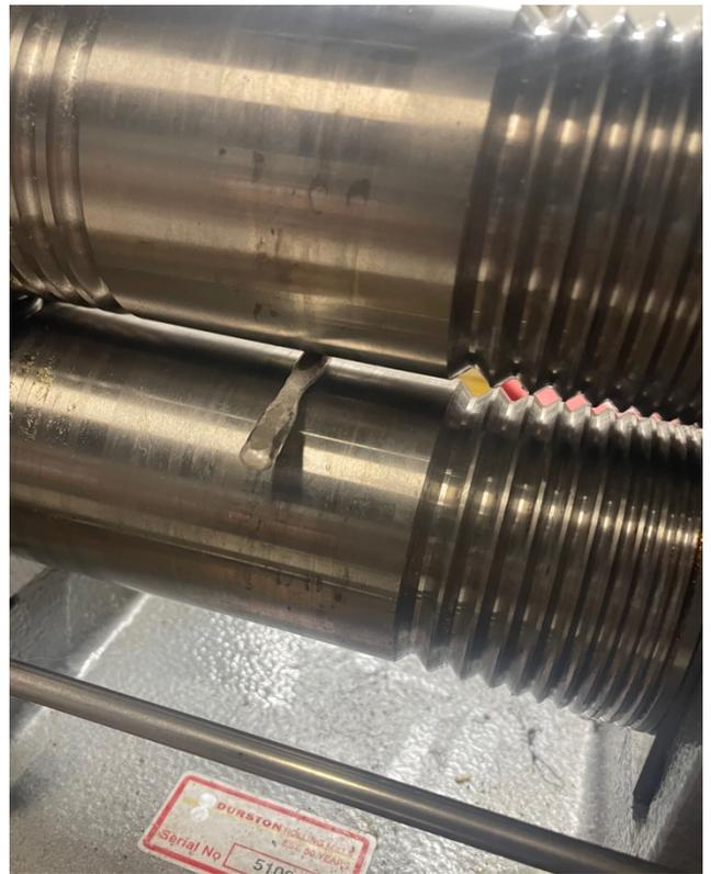
I realized the clip didn't have as much mass in the center as I wanted, so I put it back on the block and added a bit of argentium scrap to the middle to melt in.
