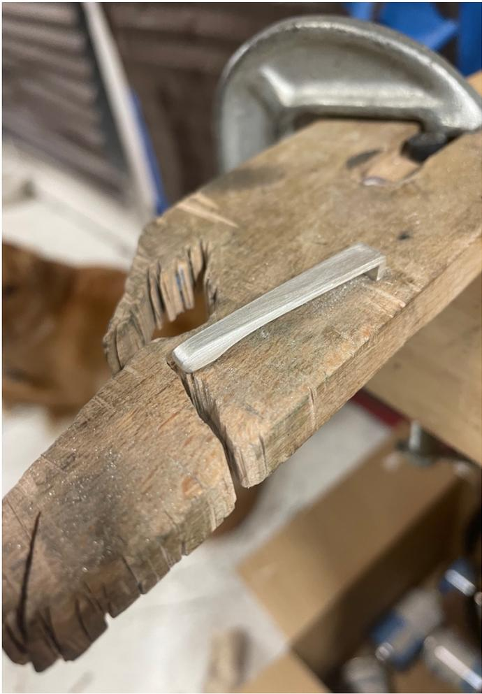
One last thing I do is take my sanding drum and form a radius on the back of the bent over part of the clip, so it conforms with the clip ring when I solder. On the block and ready to solder. I'm using a third hand and tweezers to hold the clip body in place.
