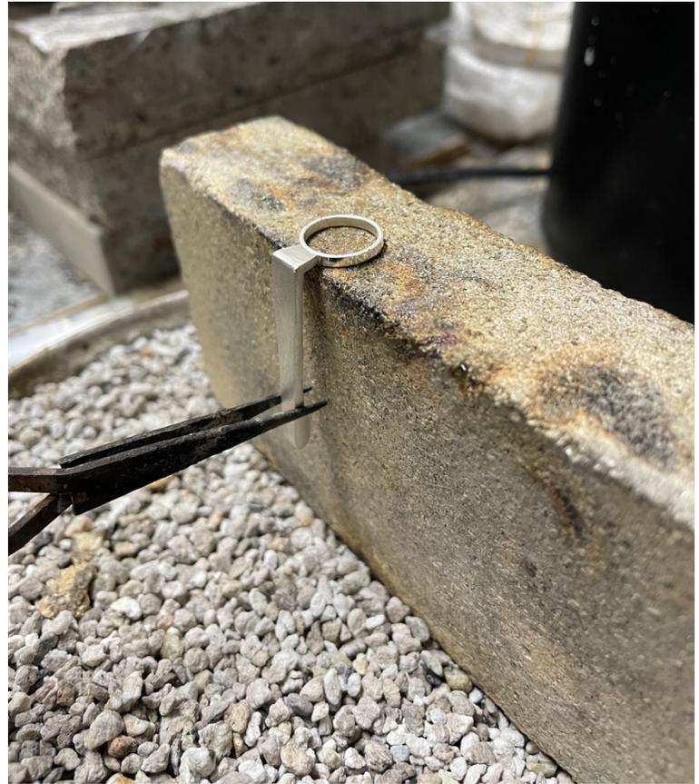
Soldered! It's important not to melt the clip ring, since it's much less mass than the clip body. I focus my torch on the body, then switch to the ring right before the solder starts to melt.
