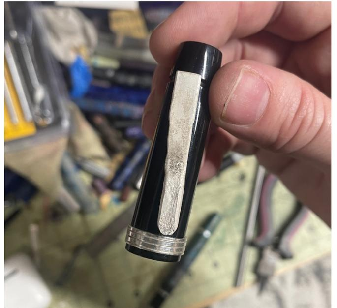
I like to use a rotary sanding drum in my freedom to blend the curve where the clip transitions into the end.
