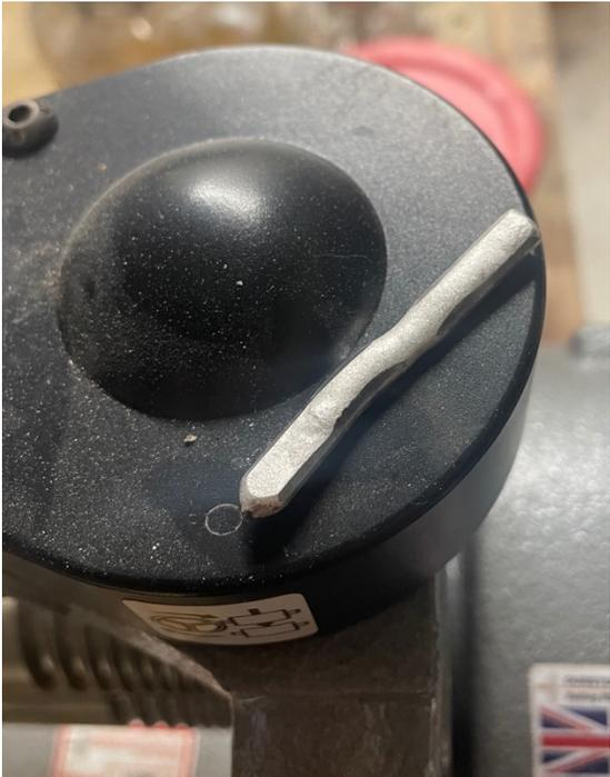
It's a bit thick at 2.65mm, so I am going to bring it down to about 1.8mm or so. Back to the rolling mill.
