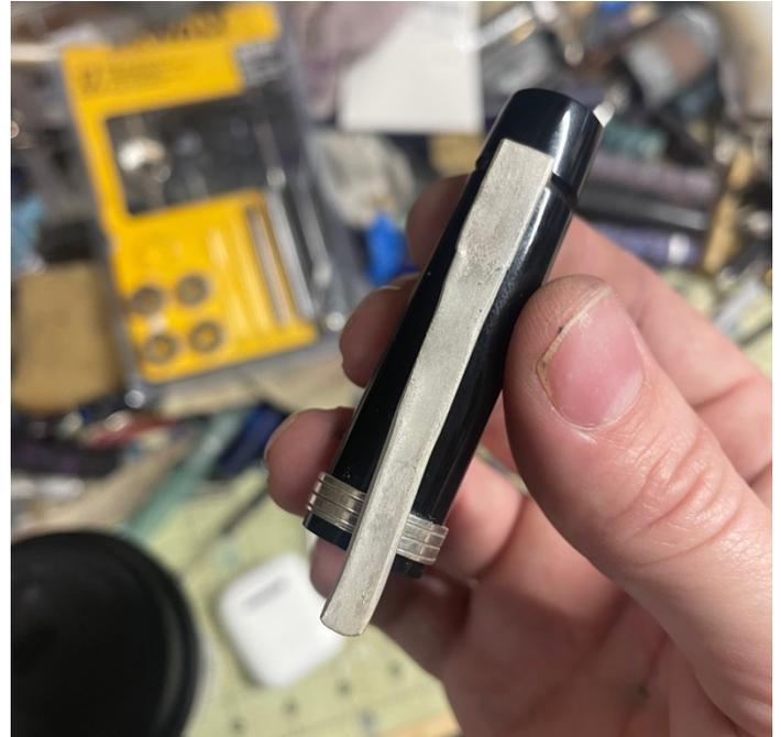
All this extra clip length will be turned into the fat part of the clip end. I put it on the soldering table and focus my heat on the end until it starts to melt, drawing the heat up the clip so the metal flows.
