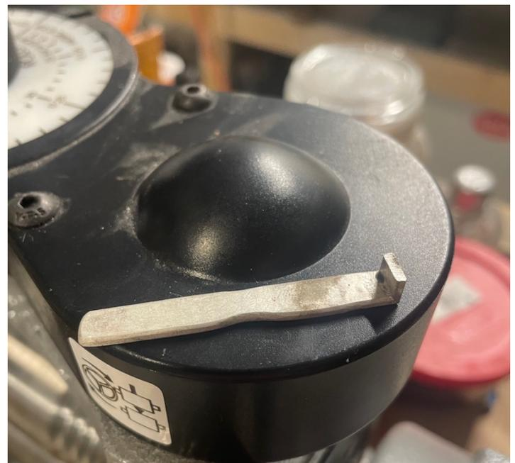
Now I want to taper the clip out. You could just saw/grind the taper, but since this is silver, I am trying to save as much waste as possible. I do this by rolling only a portion of the clip through at different roller settings. As you can see, the clip is way too long, which is good.
