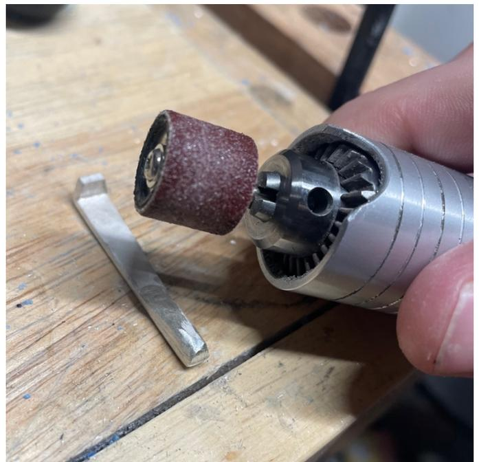
Here is the clip with the bottom filed and ready for sanding, and the top filed and sanded to about 400 grit.
