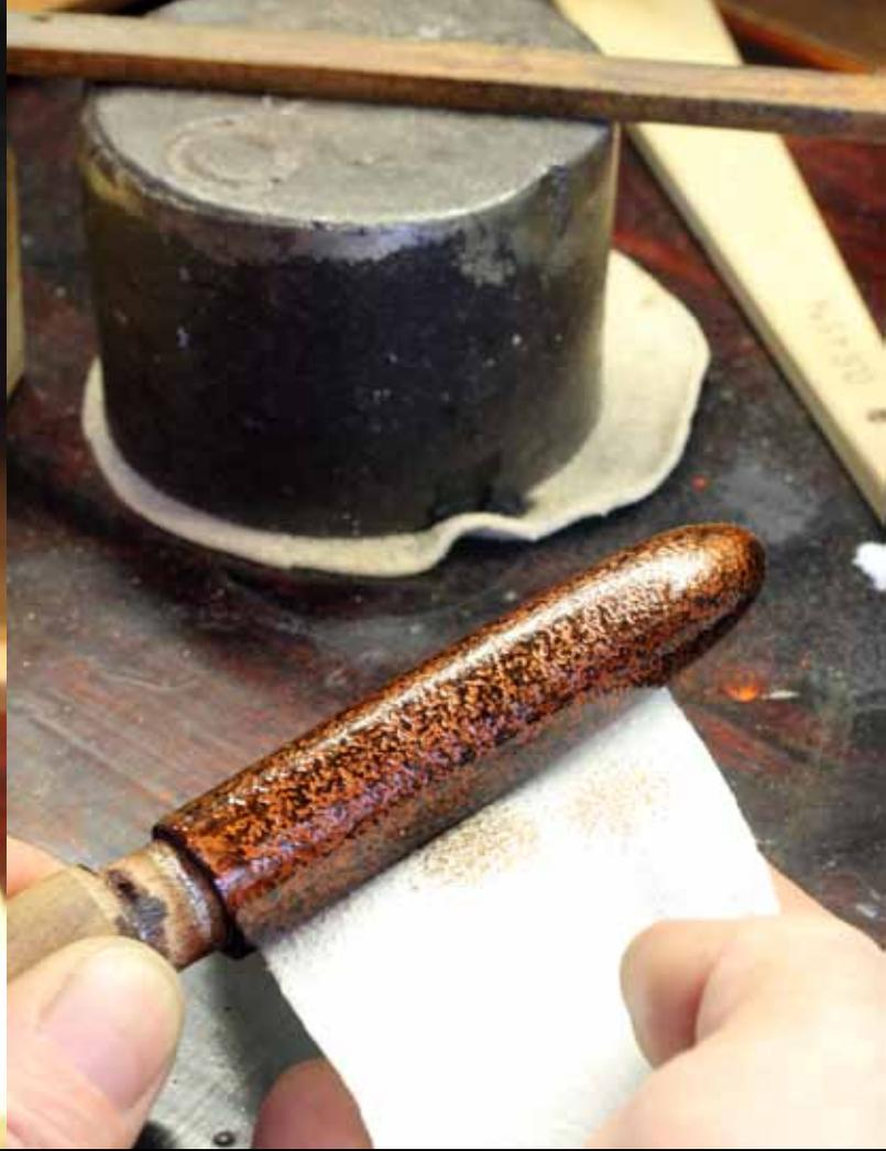
again „sugrome urushi“ is rubbed into the surface to stabilize and protect the copper powder, repeated 3 times
