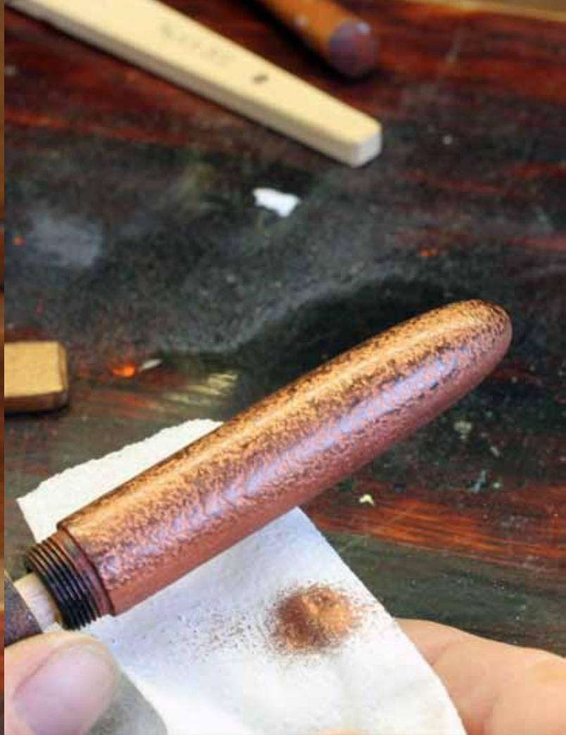
The copper powder is partially removed
