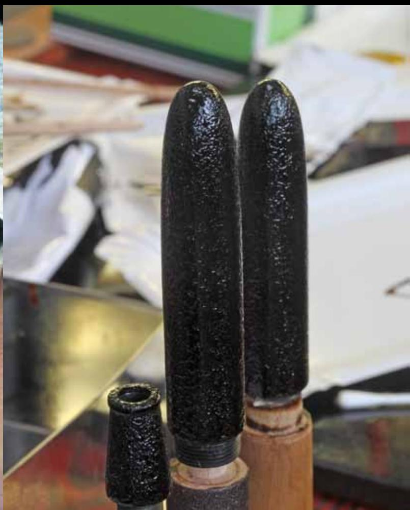
After Roiro Migaki has been done a thin coat of finest „sukurome urushi“ or „sakari urushi“ is applied and cleaned off with a paper, that little urushi only remains in the deeper sections of the surface structure
