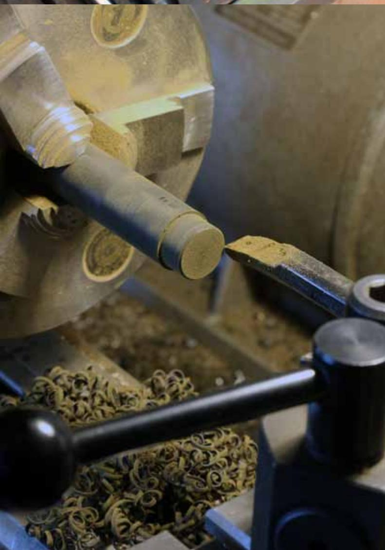
Drilling the barrel to make space for ink converter and thread
