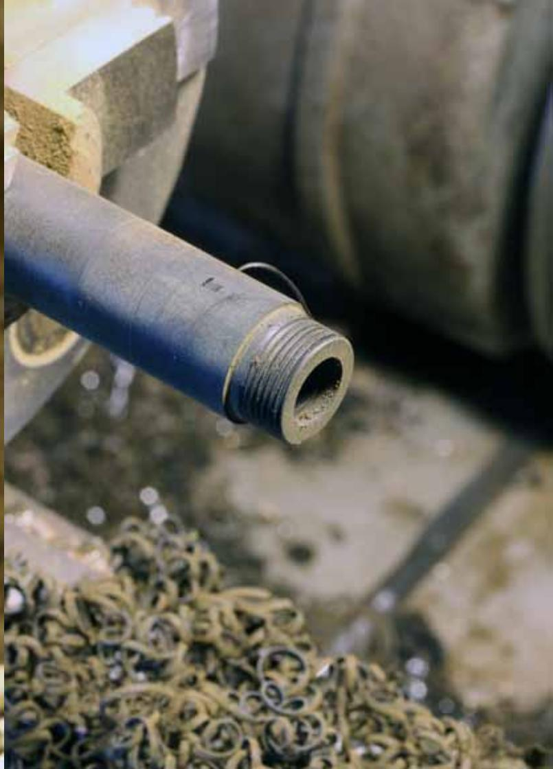
Cutting the thread for the section
