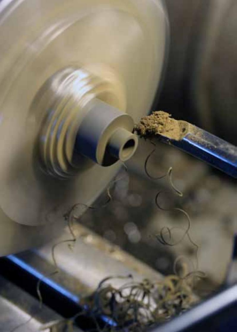
Section gets its thread to be screwed into the barrel
