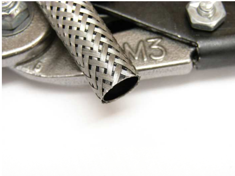
SS Cable Trimmed Just Proud of The Tube End
