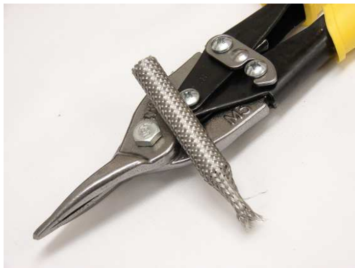
Trimming SS Cable With Metal Shears
