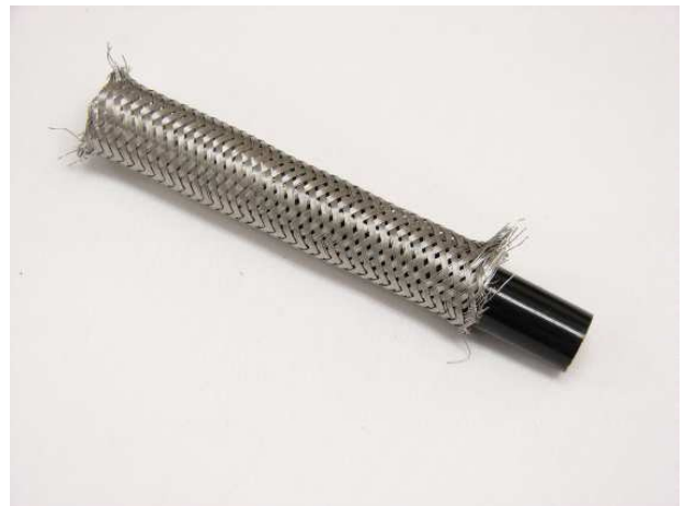
Insert Painted Tube Into SS Cable
