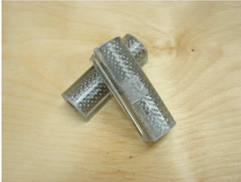
Blanks Separated from Mold Tab
