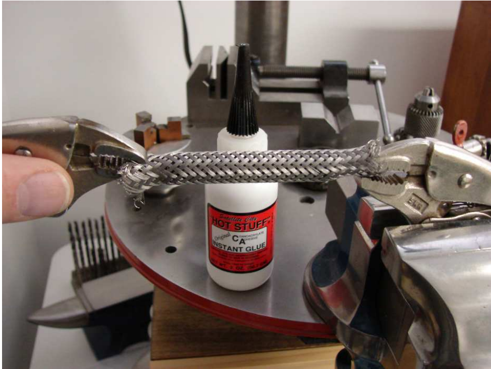
Holding Tension on the SS Cable
