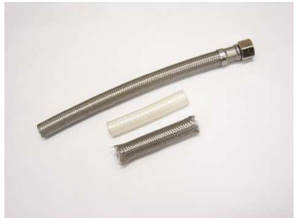
Removed SS Braid from Plastic Tubing
