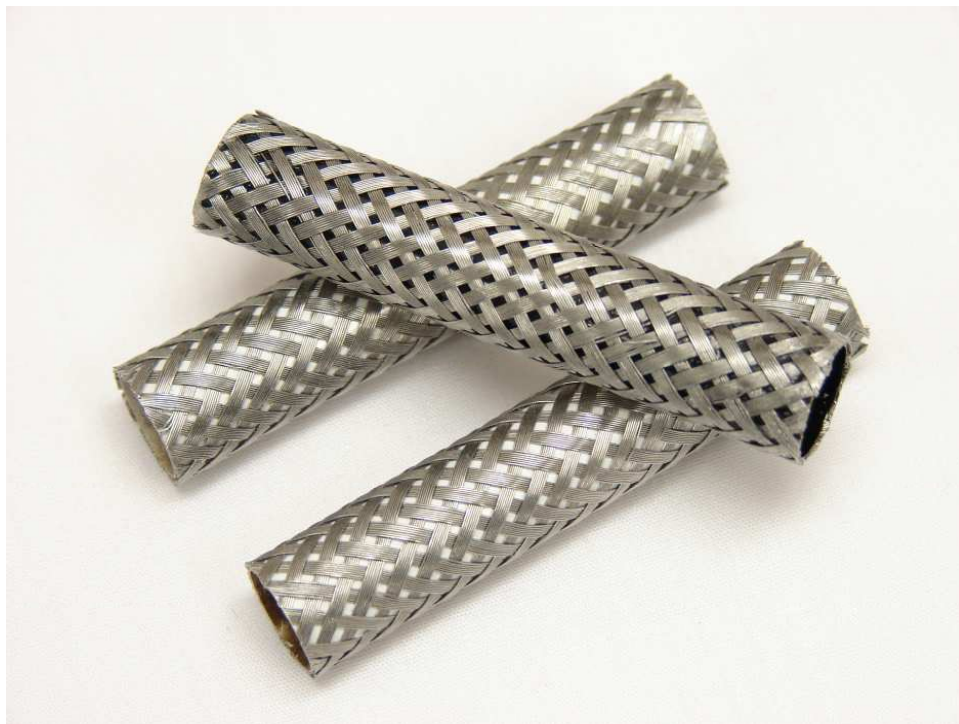
Sierra SS Cable Blanks Ready For The PR Mold
