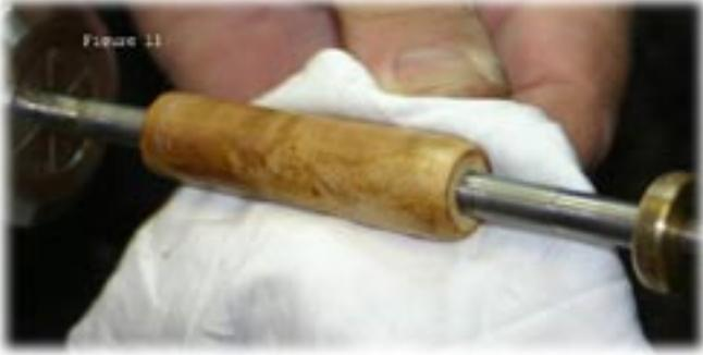
Figure 12: Application of HUT Ultra Gloss Plastic Polish. Apply on lathe and buff with a soft, dry, clean cloth. Other brands of plastic polish could be used. Some use scratch and swirl remover auto polish.
