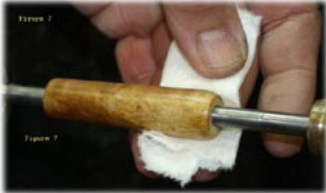
**Figure 7:** Applying the CA from the bottle. The paper towel oil applicator is underneath the blank and the CA bottle is on top. Move from one side to the other applying a bead of CA...One pass only is enough CA.
