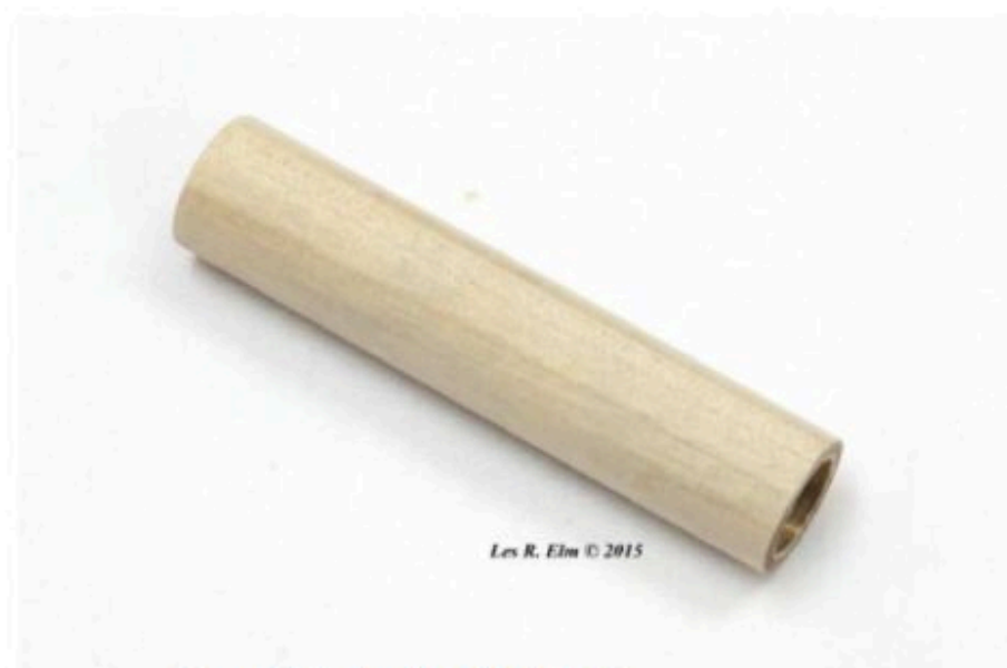
Brass Tube Anchored in Dowel
