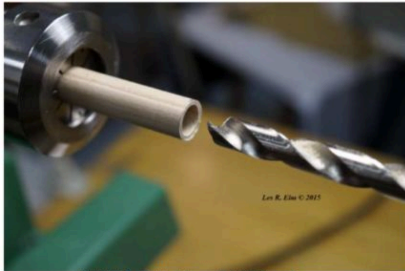
3/8" Hole Drilled through 1/2" Dowel
