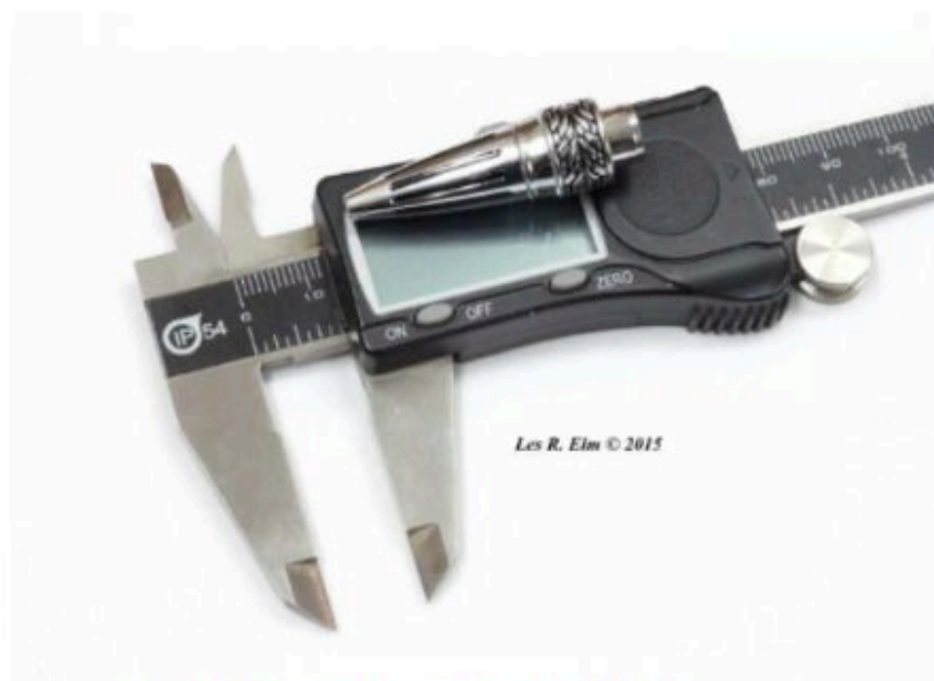
Nib Section Measurement at 0.495"
