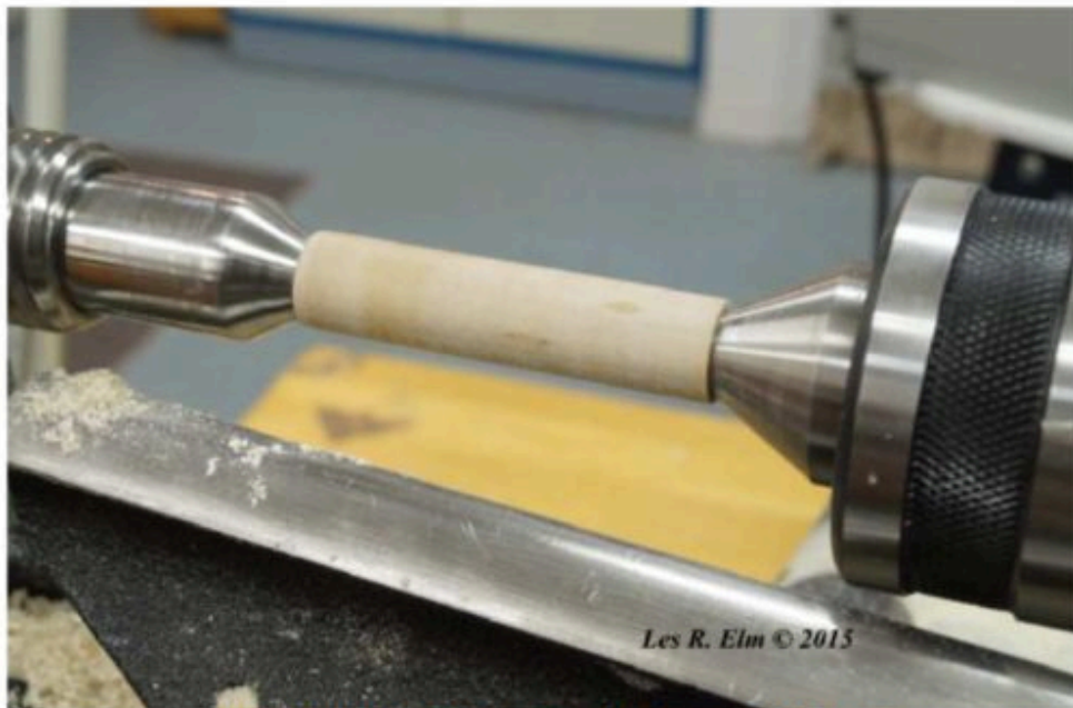
.500" Dowel Turned to Final Dimension of 0.430"
