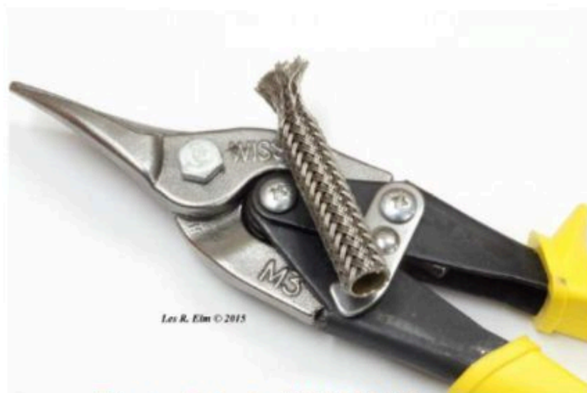
Trimming Nylon Braid With Metal Sheers
