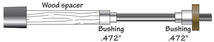
2. Advance a 60° revolving cone center into the dimpled end of the mandrel and tighten using light pressure. **Do Not** over tighten the tailstock or mandrel nut as this may cause the mandrel to flex resulting in an off-center barrel.
