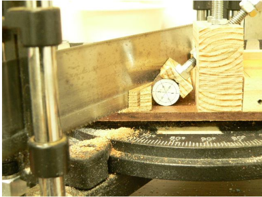
This shows the hold-down for the blank. This method applies pressure to four points on the blank
