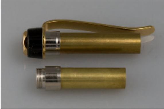
The 50BMG case is not quite long enough for the cigar pen mechanism, so it needs to be shortened. Unscrew the finial cap and remove the clip. Shorten the brass tube on the finial insert as shown in the picture to the left.
