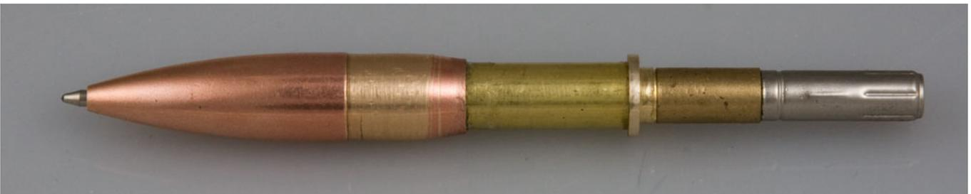
Press the modified coupler into the shortened tube and screw on the transmission. Insert the refill and test-fit the parts. With the refill extended, it should look like the above picture. If everything fits, glue the tube in place using CA glue. **Do NOT use CA accelerator.** Accelerator will damage the powder-coat finish on the bullet.
