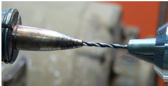
Drilling for the Cross refill
