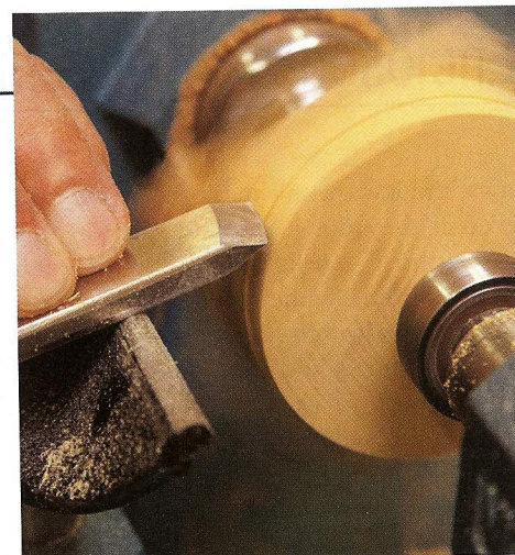
Square to round. To make the wheel blank round, take peeling cuts with a skew chisel.
