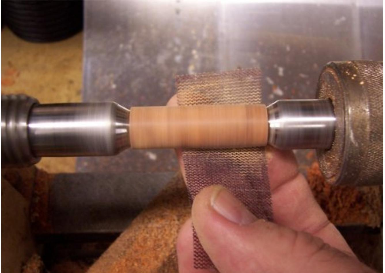
14. Since kit parts can vary from kit to kit and rather than rely on bushings, I measure the mating kit parts then check the blank to make sure it is where I want it to be. When doing a CA finish I will sand the blank slightly undersize then build up the blank with CA.
