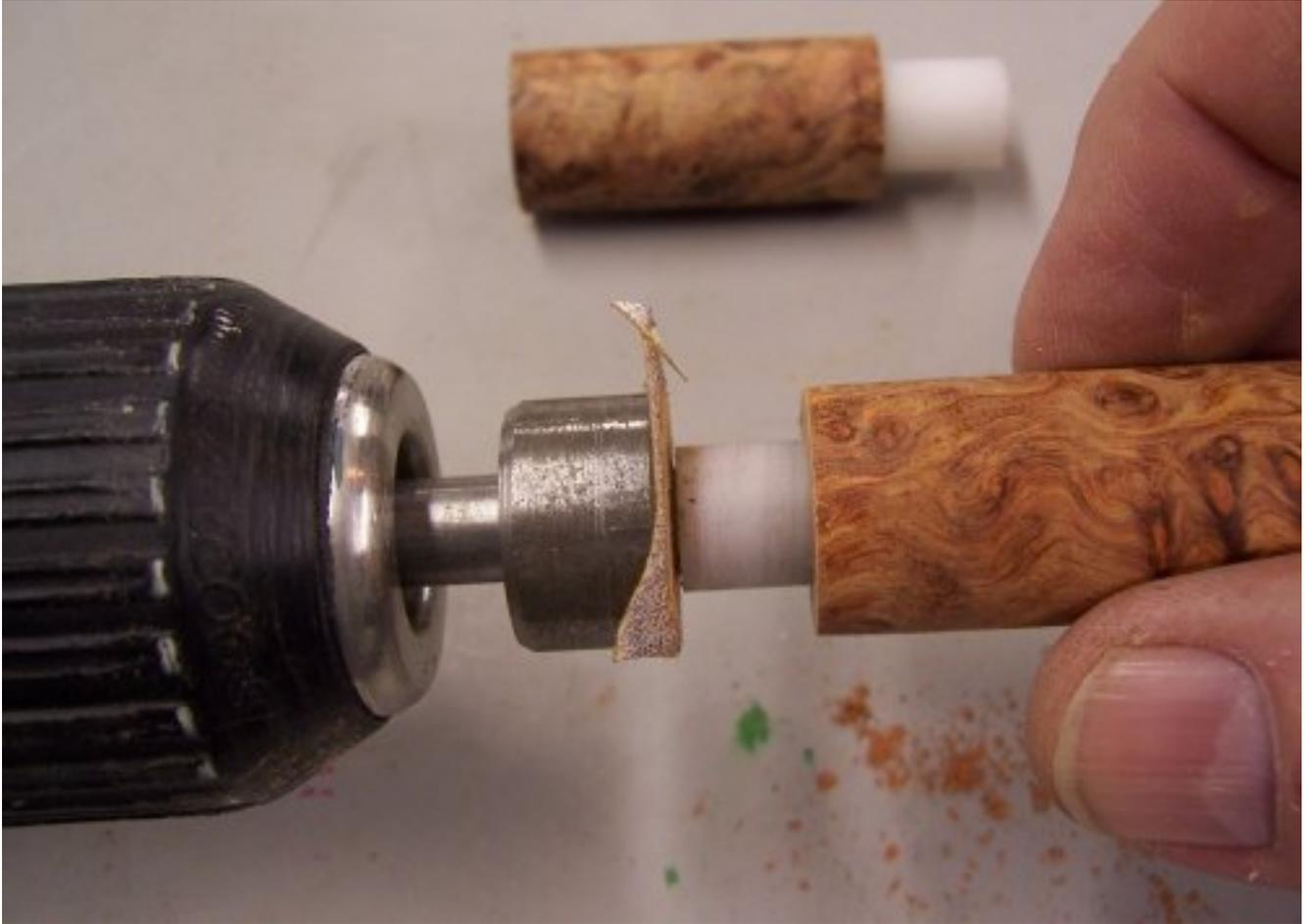
9. Now we have a squared up blank ready to mount on the lathe and turn to size. Oops, I need to remove my little bushing first!
