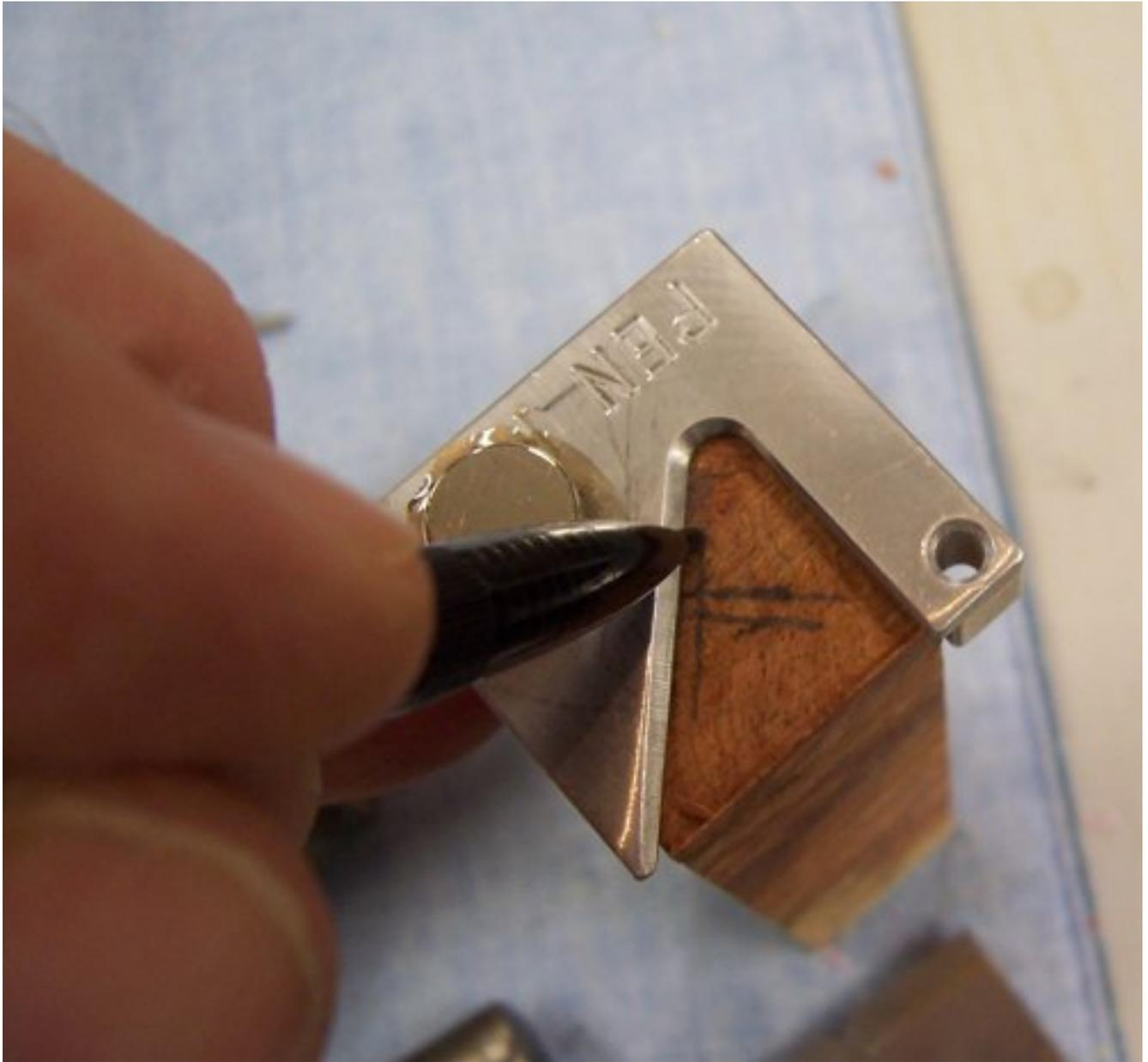
3. I use an automatic center punch to mark a dimple in the blank for the centers to zero in on.
