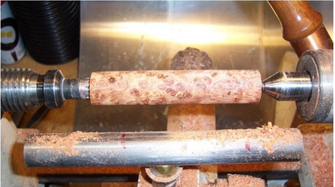
6. A benefit of rounding the blank before drilling is that I can see exactly what the pen will look like as I decide how to position the tubes before cutting. Here I decided I want the darker pattern on the cap.
