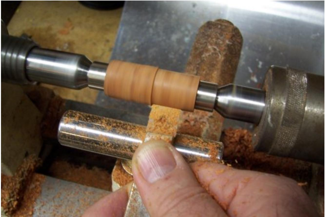
12. Here we are with the blanks turned down just proud of the bushings. The blank now comes off and we say adios the bushings.
