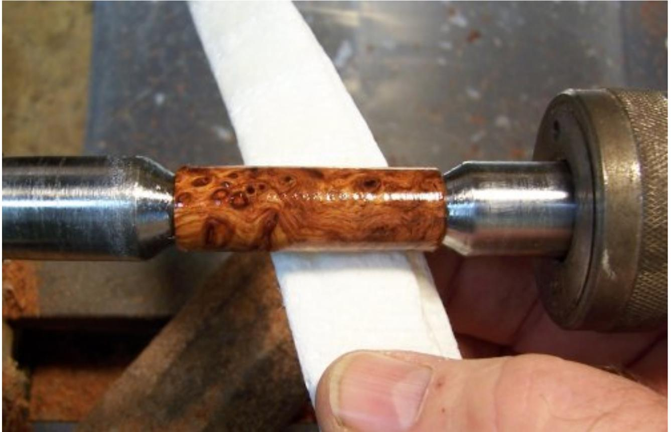
18. In my opinion, applying CA without bushings also allows CA to roll over the edge, and soaking up into the blank thus sealing the ends of the blank as well. This *MIGHT* help in the long run by keeping moisture out of the blank during actual use but has not been clinically proven! 🌱
