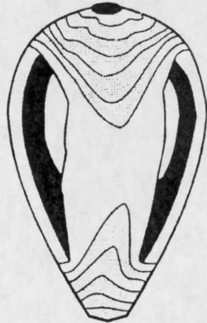
A vase form turned from a convoluted log will have openings along the sides where the wider portion of the form intersects the air.
