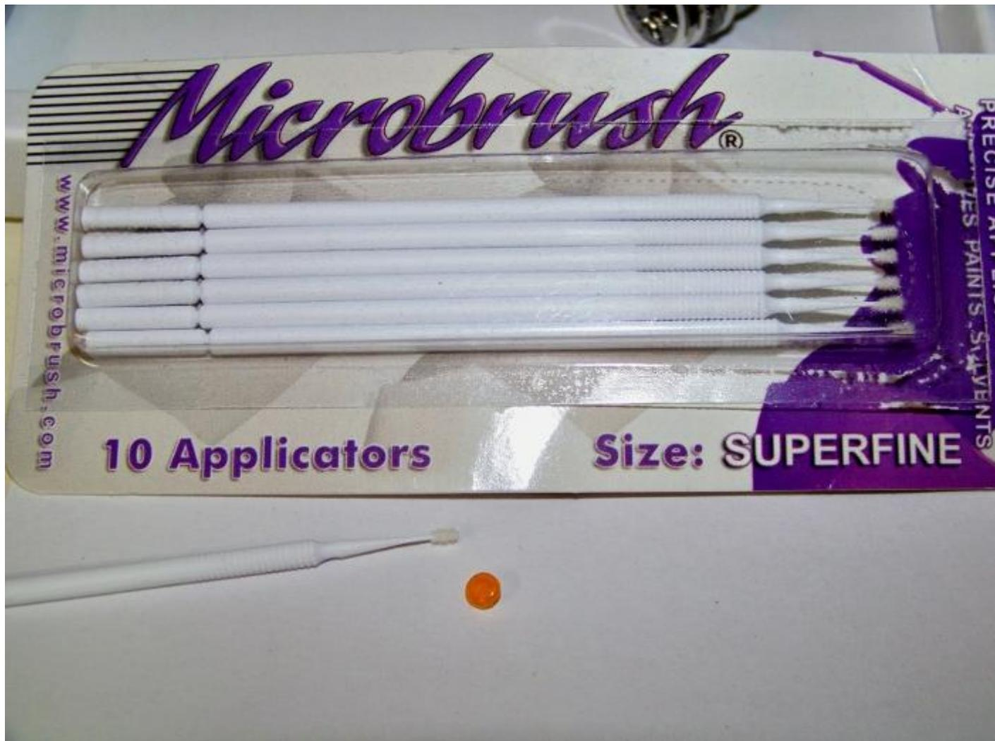
Now it's time to glue it in. I found these at hobby lobby in the model car section and are perfect for gluing small pieces. I recommend epoxy for the glue up. You have more working time and epoxy can be cleanly wiped off if there's any squeeze out.
