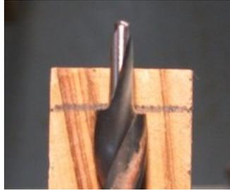
Put the mechanism in, check it for length and move the stop a little. Drill again and check. Keep doing this until you have approx. .275" sticking out. Too little and the threads won't engage, too much and you will weaken the tip. I do the fine tuning by hand with the bit in a hand vise, but if you don't have one, just leave the drill in the chuck and turn the blank by hand.
