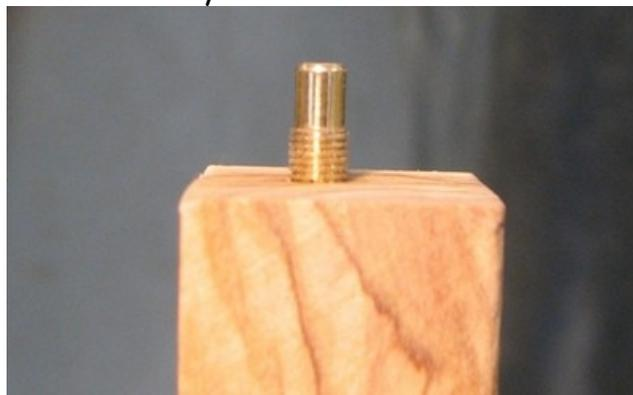
As far as the actual drilling is concerned, I like to start by using a center drill and then a regular length 17/64" drill bit to drill the first couple inches. **BY ALL MEANS** you can just use the step drill, but it tends to wobble a bit at the beginning, leaving a slightly larger hole. Also, once the flutes disappear inside the blank, don't drill any more than 1/2" at a time before backing out and clearing the flutes. 1/2" is about all it takes for
