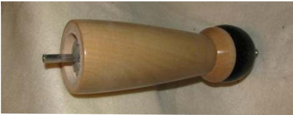
Now, screw on the threaded knob, until it is tight. Holding everything tightly together as shown above, the shaft will stick out of the bottom. Mark the shaft (a pencil line is fine, but does not photograph like the red marker did) where the grinding mechanism is “seated”.
