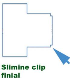
A slimline clip finial is used in "nib" the end of the barrel to accommodate the pencil mechanism. But, first the finial must be modified. The large diameter will be reduced to match the smaller diameter and then it will be step drilled for the mechanism. This modified piece will be pressed into the "nib" end. Stay tuned.
