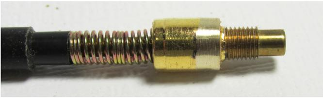
Test fit seems to be OK. I like to have about 8 threads exposed beyond the brass part for the nib to screw onto.
