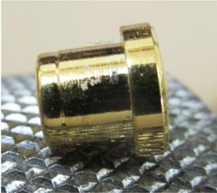
Here is a picture of the actual part that will be modified. One way to remove the larger diameter is to press the part into a brass tube and rotate it on a grinding wheel using the tube as a handle. Remove the larger (black area in the previous image) diameter until a cylinder is formed. Time to drill.
