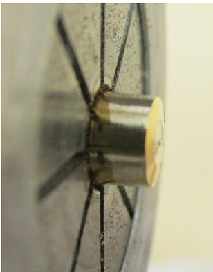
The larger diameter is reduced and the next step will be to drill this piece to accept the pencil mechanism. Leave the piece in its current place to drill the first hole. Use a center drill to make a starting hole. Then drill all the way through with a # 22 (.157) drill.
