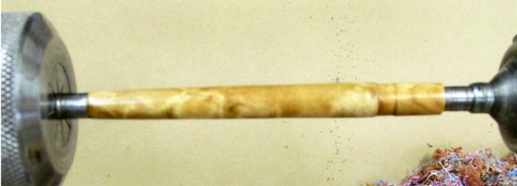
The blank is turned, sanded and a finish applied. Notice the recess on the right end for the clip. Take measurements from the original barrel. Also, did you notice I changed to standard slimline busnings and a mandrel? The longer blank was flexing being held between centers as the diameter reduced.
