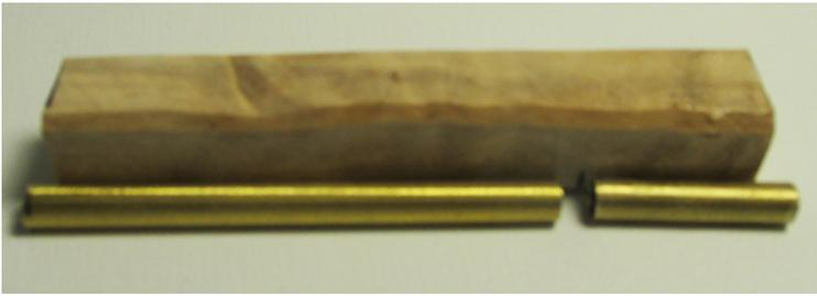
Longer 7mm tubes will be needed. 10" tubes are available. Two tubes will be needed: the longer tube is about 3.7 " long and the shorter tube is the balance of the blank's length. The longer tube is glued in place flush with one end and the shorter tube is inserted in the other end. It is NOT glued in the blank.
