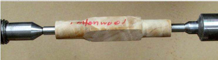
The blank is mounted with between center bushing between a dead center and live center.
