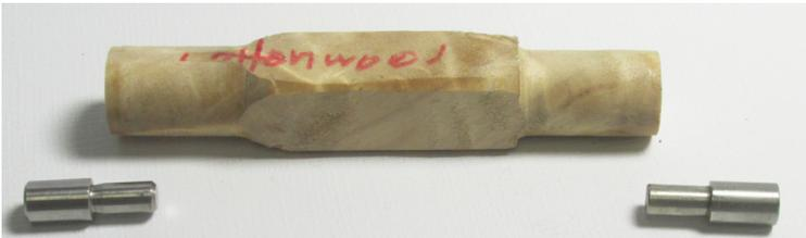
After the tubes are inserted square both ends tuning the blank to the correct length. I plan to turn the blank between centers using these two between center bushings holding the blank between a dead center and a live center;
