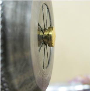
The clip finial held in a PSI collet chuck with a 1/4 inch collet. Use a parting tool to remove the larger diameter. This part is brass so removing material will be quite easy. Just go slow, taking light cuts but a fast speed seems to be best. Be sure to faced the slightly domed surface.
