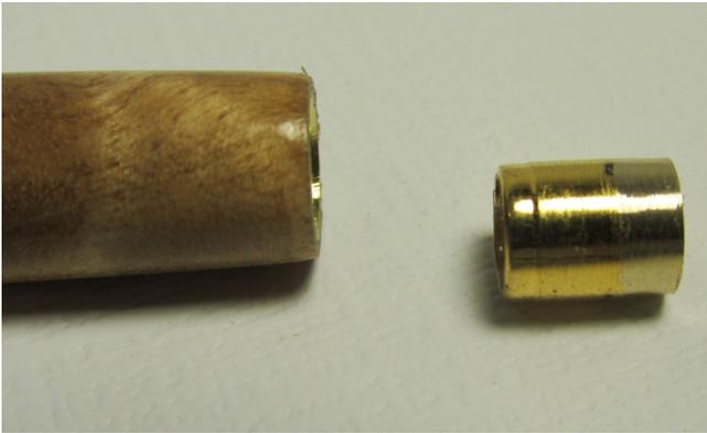
This piece is ready to be pressed into place. Pay attention to the orientation of the piece with pressing it in. The larger diameter hole should enter the pen blank first. But, it can be removed and pressed in the correct way if needed. DAMHIK!
