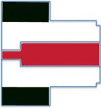
The black will be removed and the drilling will form the red shaded area.. I hold the clip finial in a collet chuck but other methods can be used. Possibly a jacob's chuck will work to hold the piece. DO NOT USE A JACOB'S CHUCK IN THE HEADSTOCK WITHOUT A DRAWBAR.
