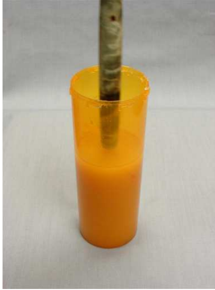
Dipping Blank Into MINWAX
