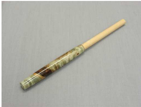
Wooden Dowel Inserted Into Blank End
