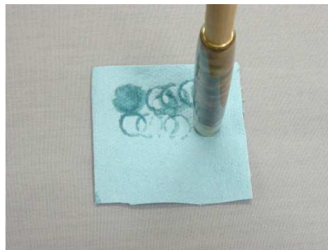
Wicking MINWAX From Blank End
