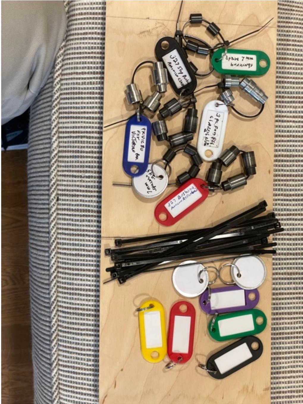
For pen turners one of the most irritating tasks is to label and keep track of the bushing sets that are used to turn a pen barrel to the correct dimensions . The bushing sets vary from two to four pieces per set. The individual bushing pieces are small, and there is essentially no space on the bushings themselves for an identifying label.
