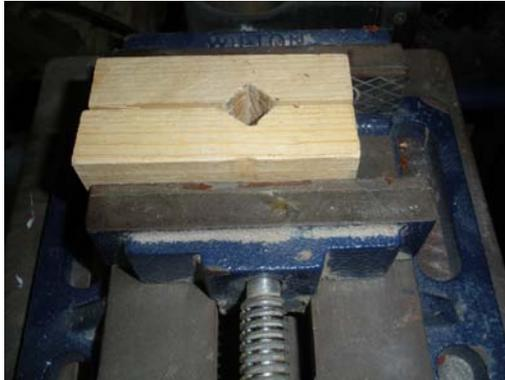
8. Drill hole  $3/16^{\text{th}}$ " deep and add slit down side of the holder just a tad longer than the width of the smaller diameter's hinged "wing."
