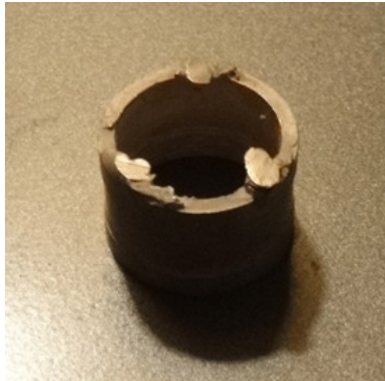
Center band with sprues needing filing
