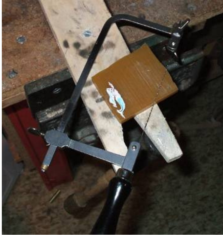
Cutting out pattern with jeweler's saw
