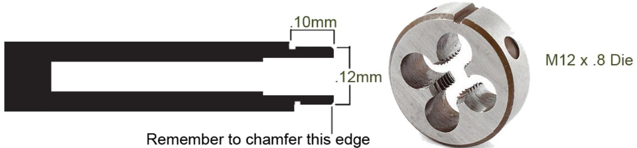
This part of the cap end can be recessed with a drill bit to accommodate the clip.
