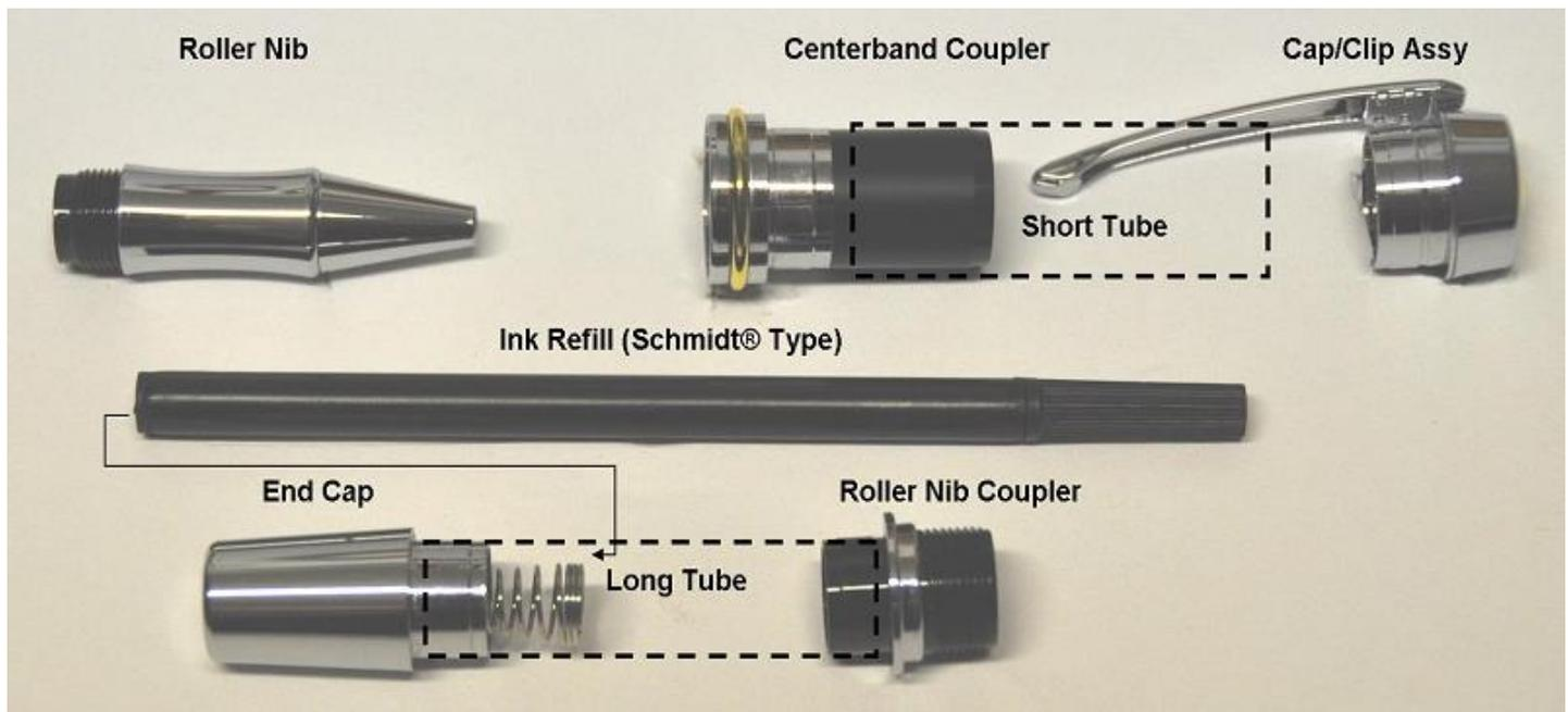
1. Press the end cap and threaded coupling into the opposite end of the long tube.
