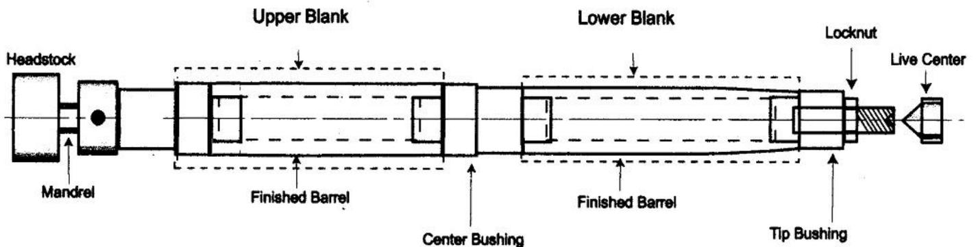
After aligning the bushings and blanks, thread the lock nut and hand tighten. The turning unit should now be secure on the mandrel. Slide the tail stock over and set in place next to the mandrel, ensuring there is enough pressure to secure the mandrel (do not over tighten or the mandrel and live center could be damaged). Turn the blank down to the approximate diameter of the bushings and then sand to the desired finished diameter.
