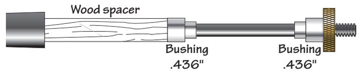
2. Advance a 60° revolving cone center into the dimpled end of the mandrel and tighten using light pressure. **Do Not** over tighten the tailstock or mandrel nut as this may cause the mandrel to flex resulting in an off-center barrel.
