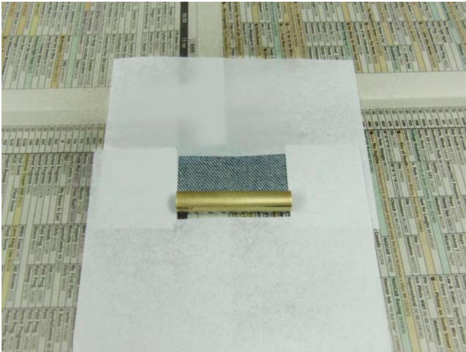
Spray the cloth and tube with spray adhesive. Go easy, do not spray too much. Put on your rubber gloves and roll the tube up the cloth.
