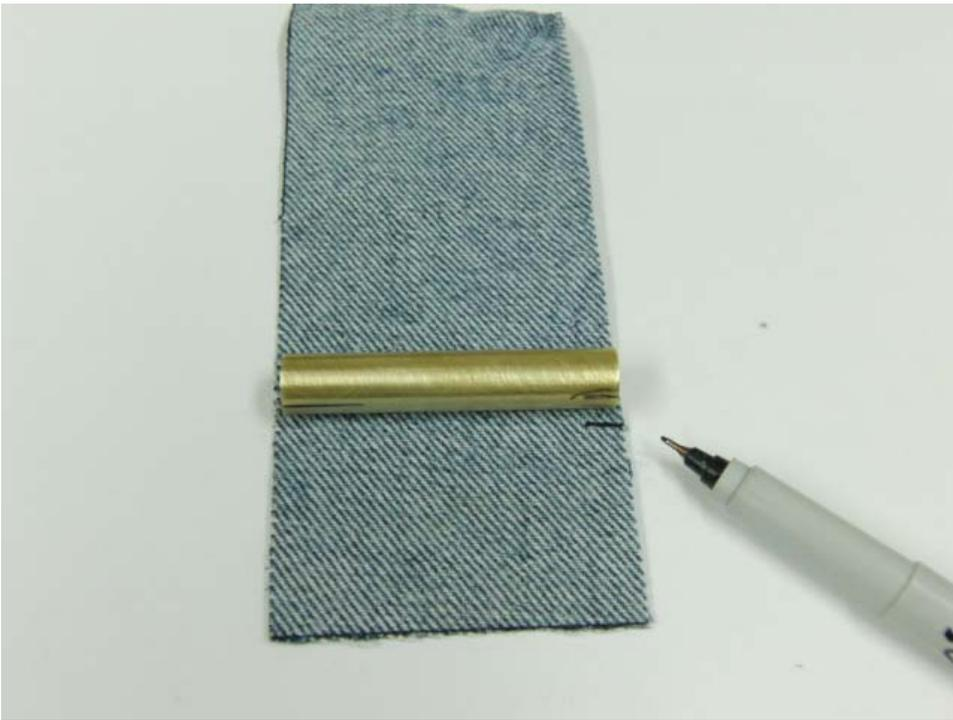
After you roll the tube up the cloth and see the marks on the tube (again), you know you have enough material to wrap around the tube. But, but ... give it another 1/8" extra for trimming later.
