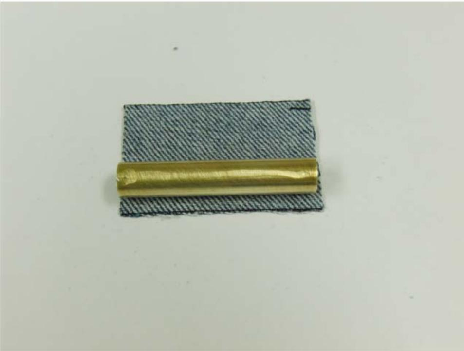
I hope you can see a line of thick CA on the tube. Now roll the tube back toward you/toward the near edge. Hold it for a few seconds.
