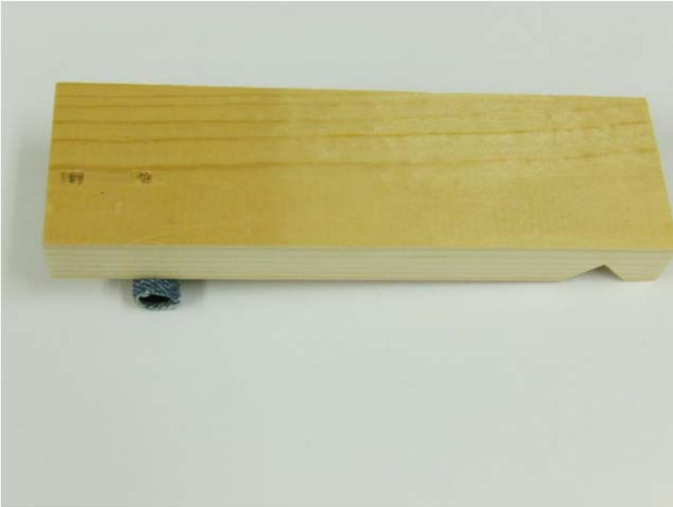
Use a piece of softwood to roll the tube (gently) to make sure the glue has good contact.
