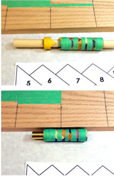
Remove the assembled kit from the dowel and slide a tube inside the kit. The tube is shorter than the assembled kit so you can place the assembly in a vice to compress the pieces together while you apply the final tape.
