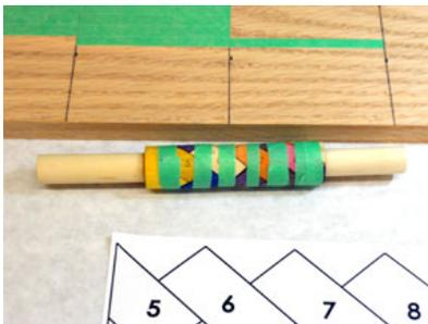
After the pieces are all assembled except for #19 and #20, remove the tape from the end assembly jig, slide the assembled pieces away from the jig and install and tape the last two pieces.
