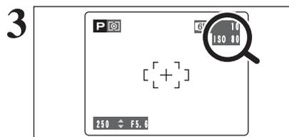
When the sensitivity is set to "80", "100", "200", "400" or "800" the selected sensitivity setting appears on the LCD monitor.
