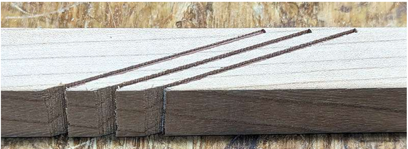
The first 3 inserts are in place and ready for CA
