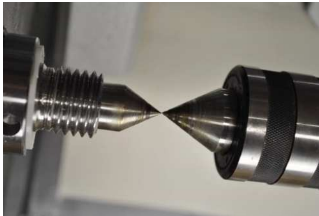
Dead Center and Live Center Points Lined Up
