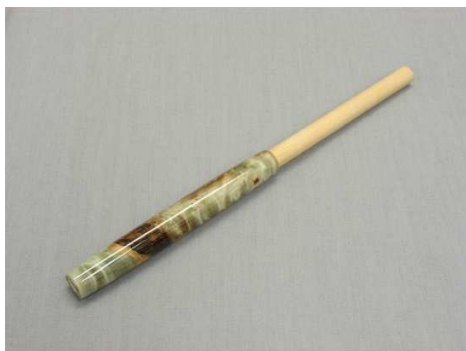
Wooden Dowel Inserted Into Blank End
