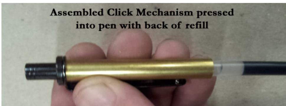
9. At this point you have to press the two barrels together with the fully assembled mechanism plus the refill and smaller spring inside the pen. The mechanism must remain in the “retracted position” during pressing. In order for this to occur you need to press the two sides together without pushing on the plunger. There are three ways to do this.
