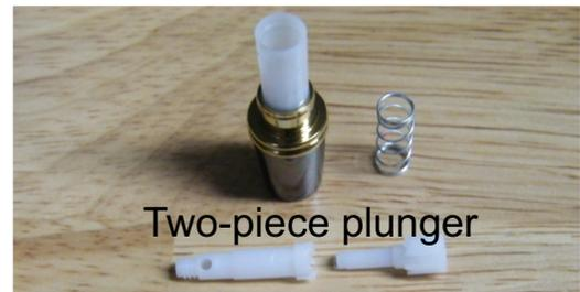
Take the lower piece of the two-piece plunger and push it into the upper piece (threaded with hole). Using a tweezer or some other device, push the assembly through the plastic sleeve that is now glued to the metal top. You may have to rotate these parts until they can be easily inserted, do NOT FORCE them!!! From the top, put the spring over the threaded plastic piece and then screw on the metal, plated plunger.
