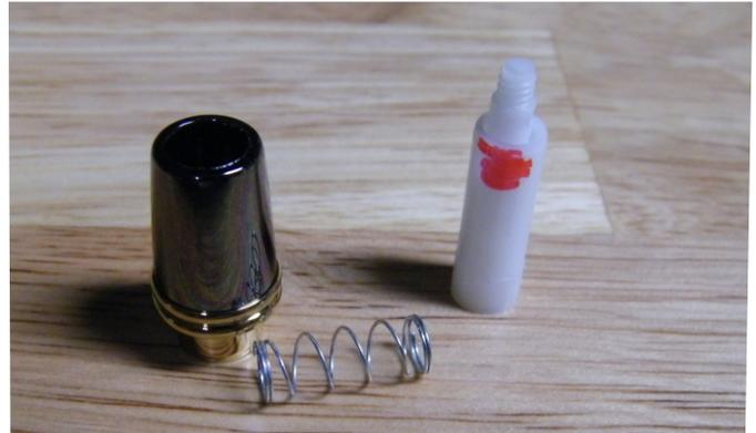
Now insert the white sleeve into the bottom of the metal cap assembly, the marked end should be inserted, so it looks like the picture, here. Put a little locktite (do not use CA glue) on the white piece, so it is adhered to the metal piece. Set aside for a day to cure.
