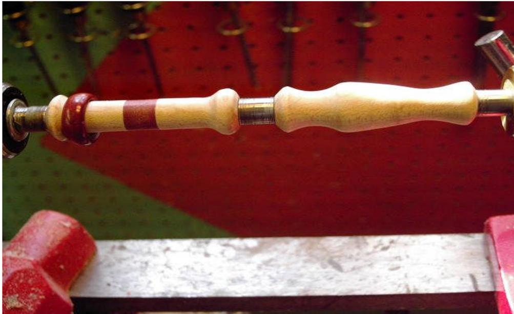
Now finish by straightening the shaft where the ring is and finish the bottom of the pen as you see fit.
