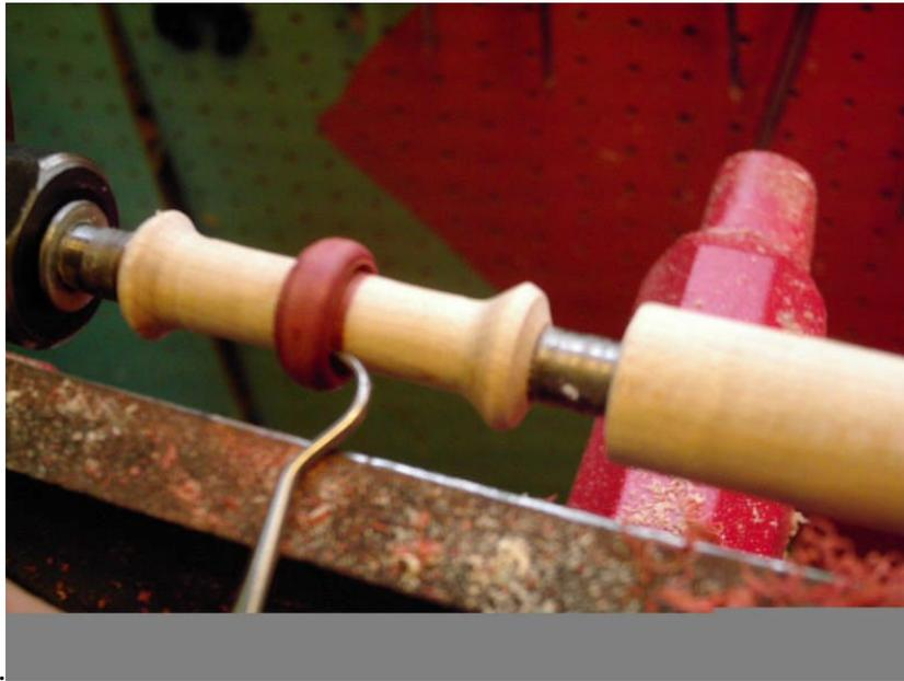
Now the fun begins. I turn the lathe down a notch to cut. Round over the ring and size it.
