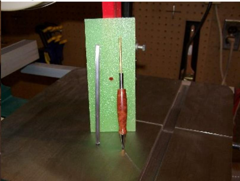
A sharp smack on the brass rod will remove the nib, as shown in Figure 3.
